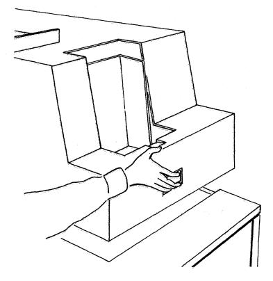
2 Release the operator panel by pressing the latches on the left and right sides of the panel once. Pivot panel to the front.
