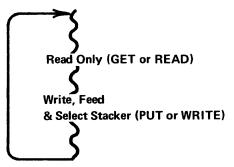
Punching into Prepunched Cards: This file type (that is, sequence of commands) should be used whenever you are punching data into prepunched cards, because the read-punch command sequence causes the subsystem to suppress the punch retry function for punching errors. If the punch retry function were not suppressed, and if a punch error were to occur, the subsystem would automatically try to punch data correctly into the following two cards.
