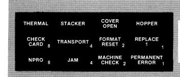
If indicators are not in a combination shown on any error display, or if an operator recovery action is unsuccessful, treat the condition as a permanent error and perform the procedure specified by the source program.
