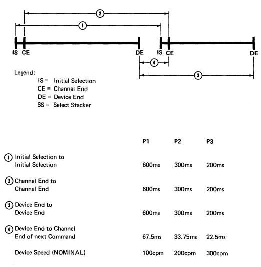
*Note:* The time between initial selection and channel end of a Write, Feed, Select Stacker command is a function of the time required for a complete data transfer.
