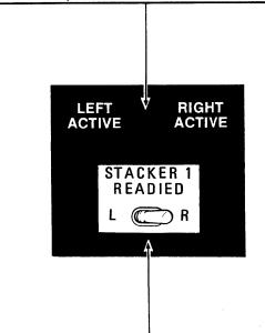
The readied toggle switch, which is set by the operator, indicates that a stacker is ready to receive cards after the active stacker becomes full.
