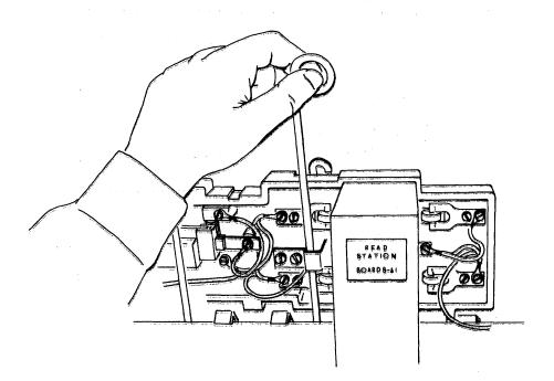
Access the post-read station by pulling the lever on the post-read station cover toward the back of the machine. (Although shown in this drawing from the rear of the machine to show machine details, accessing is usually performed from the front.)
