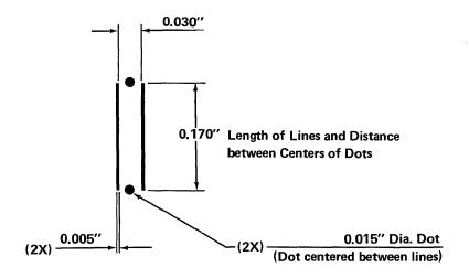
*Note:* Marking restraints (which are shown as dots and vertical lines on this drawing) must be printed in reflective ink.
