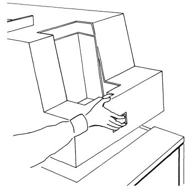
2 Release the operator panel by pressing the latches on the left and right sides of the panel once. Pivot panel to the front.
