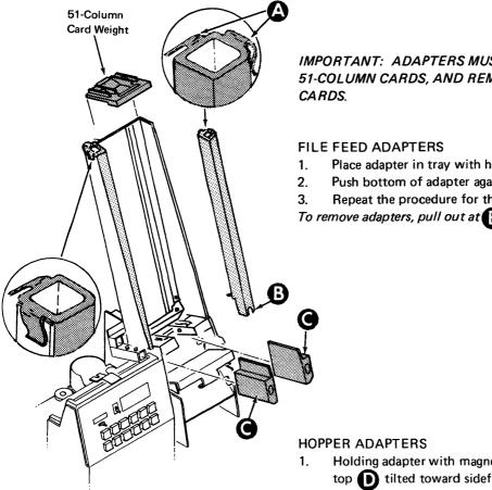
IMPORTANT: ADAPTERS MUST BE INSTALLED TO PROCESS 51-COLUMN CARDS, AND REMOVED TO PROCESS 80-COLUMN
