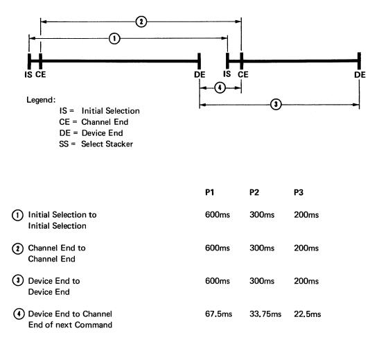
*Note:* The time between Initial Selection and Channel End of a Read, Feed, Select Stacker command is a function of the time required for a complete data transfer.
