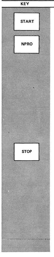
Turns on the motor and runs cards into the machine and/or establishes a ready condition. During error procedures, pressing this key resets the stop indicators and error circuits if the condition causing the error indication has been corrected.
