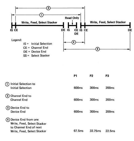
*Note:* The time between Initial Selection and Channel End of a Read Only or a Write, Feed, Select Stacker command is a function of the time required for a complete data transfer.
