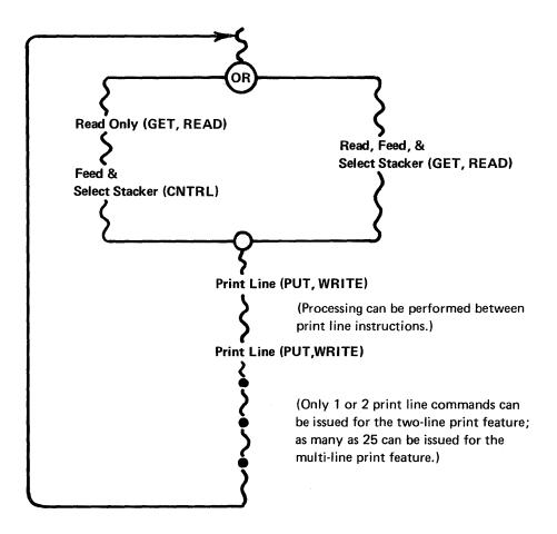
If preselection of the card is possible, then the read, feed, and select stacker command is suggested for this application. If the card is to be stacker-selected by means of data read from the card, the program should issue a read only command, process the data, then issue a feed and select stacker command specifying the appropriate stacker.
