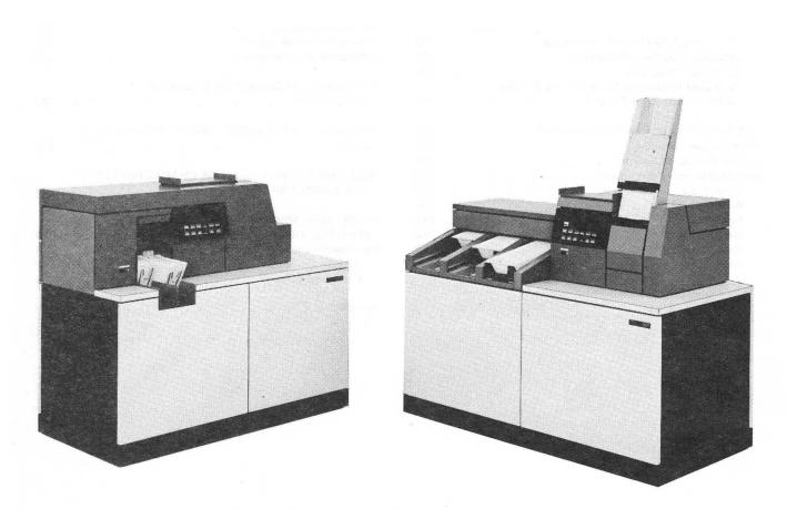
IBM 3525 CARD PUNCH WITH AN IBM 3504 OR 3505 CARD READER
