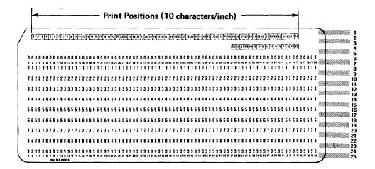
The last two lines of data to be printed are printed in an overlap mode — that is, these lines are printed during the next card feed cycle. Each print line is 64 characters long, with ten characters to the inch horizontal spacing. Maximum throughput when printing (in cards per minute) depends upon the machine model, the average number of lines being printed, and the location of the printed lines.
