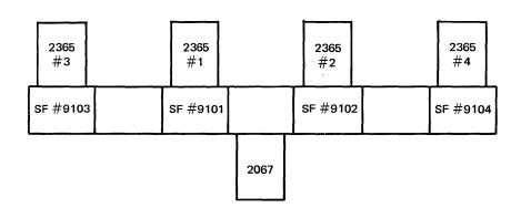
Example 15–SF #9104 attaches 2365 Model 2 #4 to 2067 Model 1 (2365 Model 2 with SF #9103 is a prerequisite).
