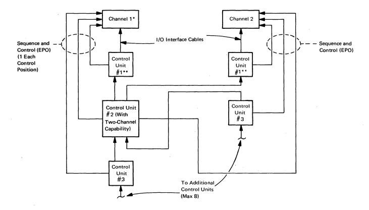
\*The channel may be a separate unit (such as the IBM 2860) or integral to the system processing unit. \*\*Units with two-byte interface feature must be installed first on the channel.
