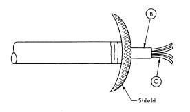
Step 6: Carefully lay the shield back over the cable outer jacket; wrap tape around the shield for temporary protec-
