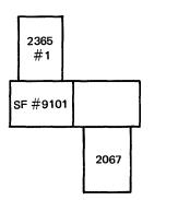
Example 12–SF #9101 attaches 2365 Model 2 #1 to 2067 Model 1.  $\checkmark$
