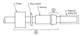
Slide the brass washer over the shield and up against the mating surface of the bushing at (F). Wrap tape around the shield for one full turn and trim off the remaining shield strands. Install the clamp and be sure that the mating surface is tightly against the brass washer.
