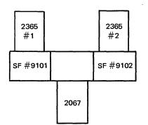
Example 13-SF #9102 attaches 2365 Model 2 #2 to 2067 Model 1 (2365 with SF #9101 is a prerequisite).
