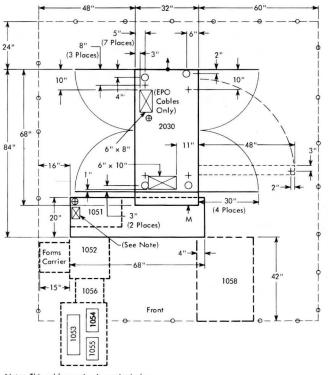
Note: This cable opening is required when SF # 3622 or 1051 is installed.
