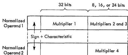
Proceeding from right to left through the multiplier or multipliers, underline from each two adjacent one bits (including these) to the next leftmost two adjacent zero bits (excluding these). For example:
