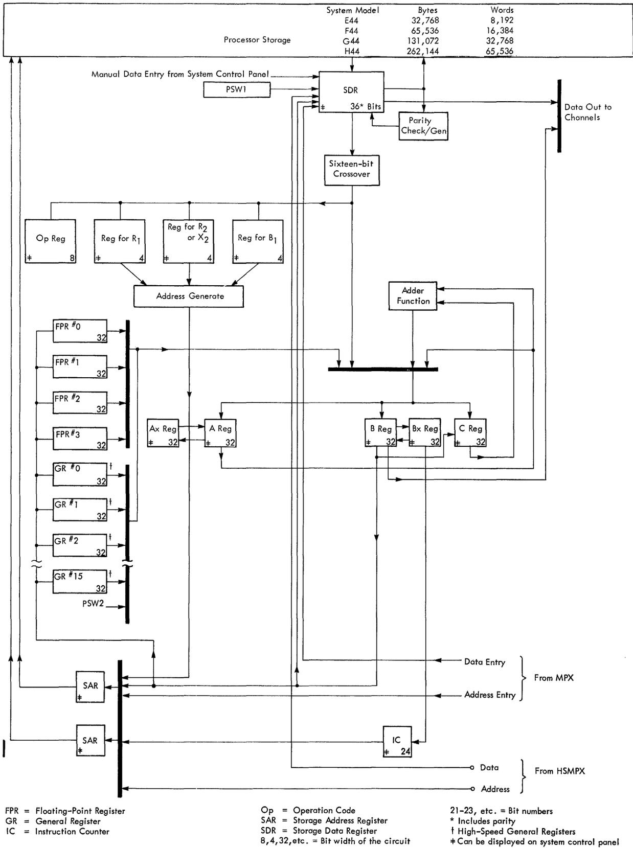
Figure 3. Data Flow in Model 44 CPU
