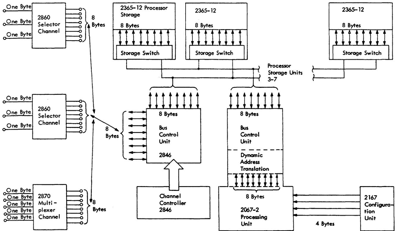
Figure 12. Model 67-2 Data Flow Diagram
