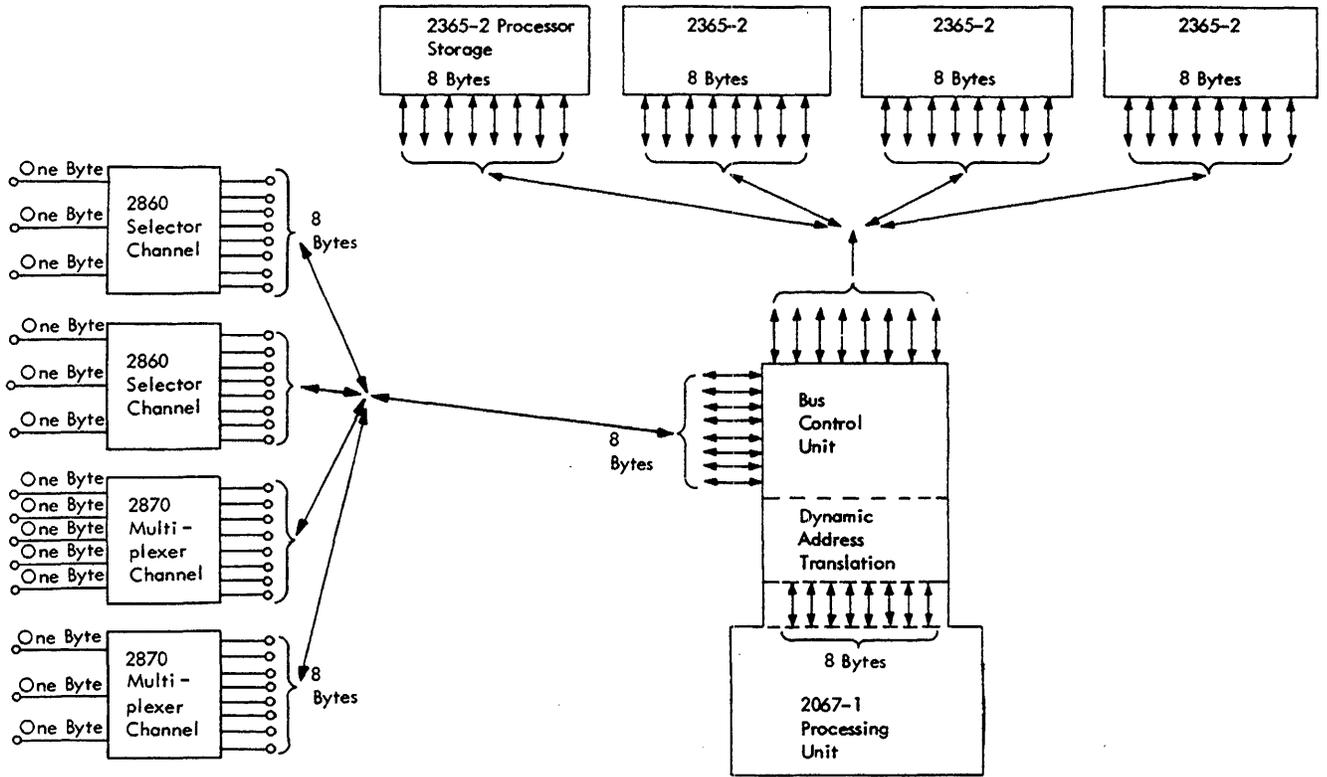
Figure 11. Model 67-1 Data Flow Diagram
