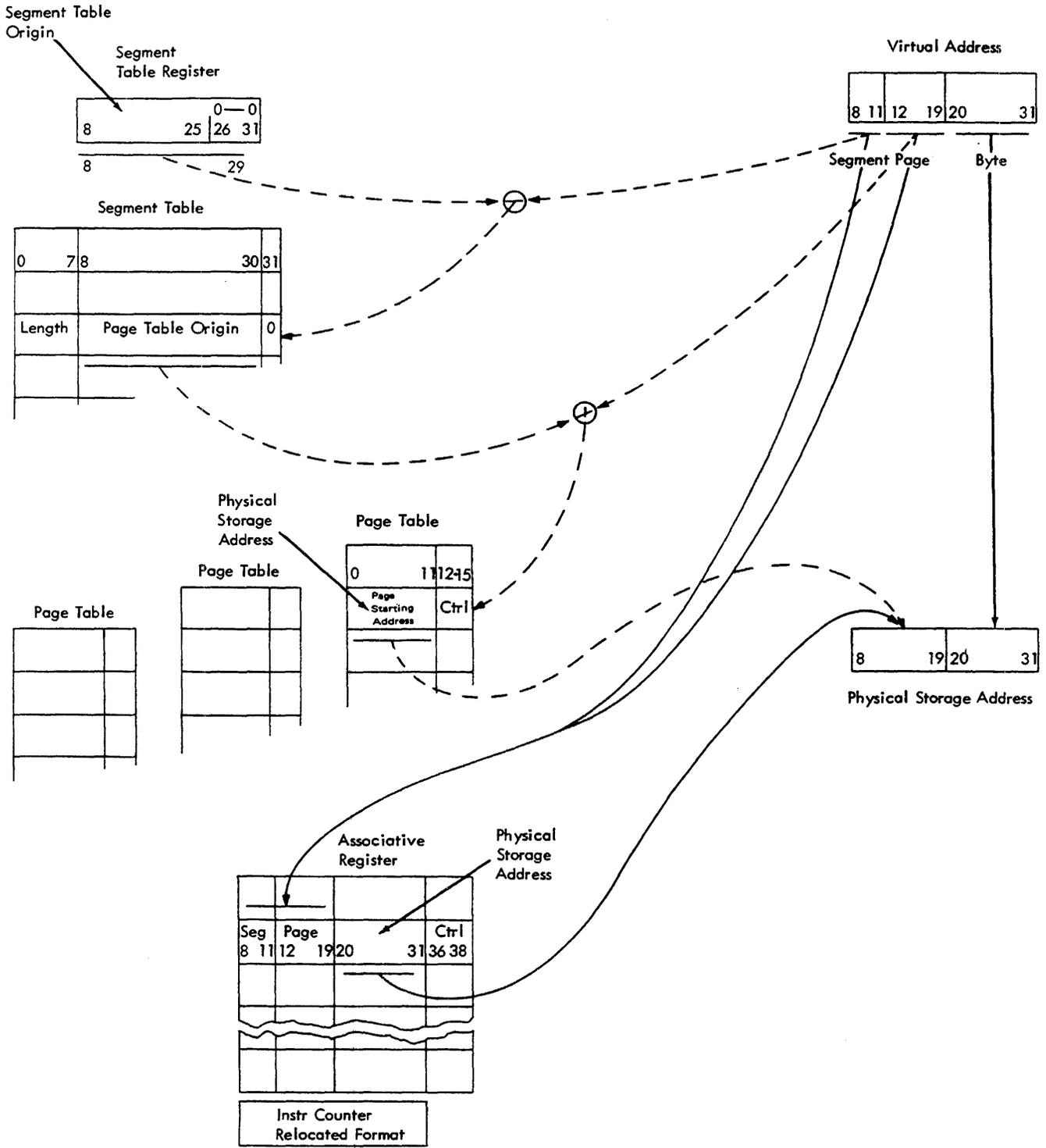
Figure 5. Data Flow for Dynamic Address Translation (24-Bit)
