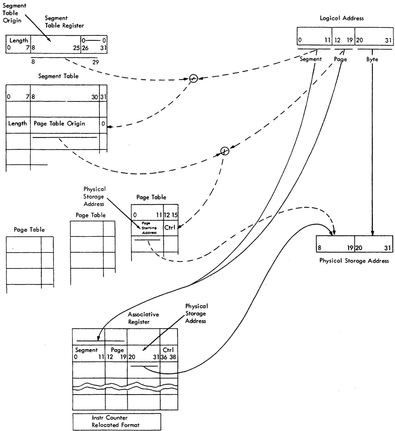
Figure 6. Data Flow for Dynamic Address Translation (32-Bit)
