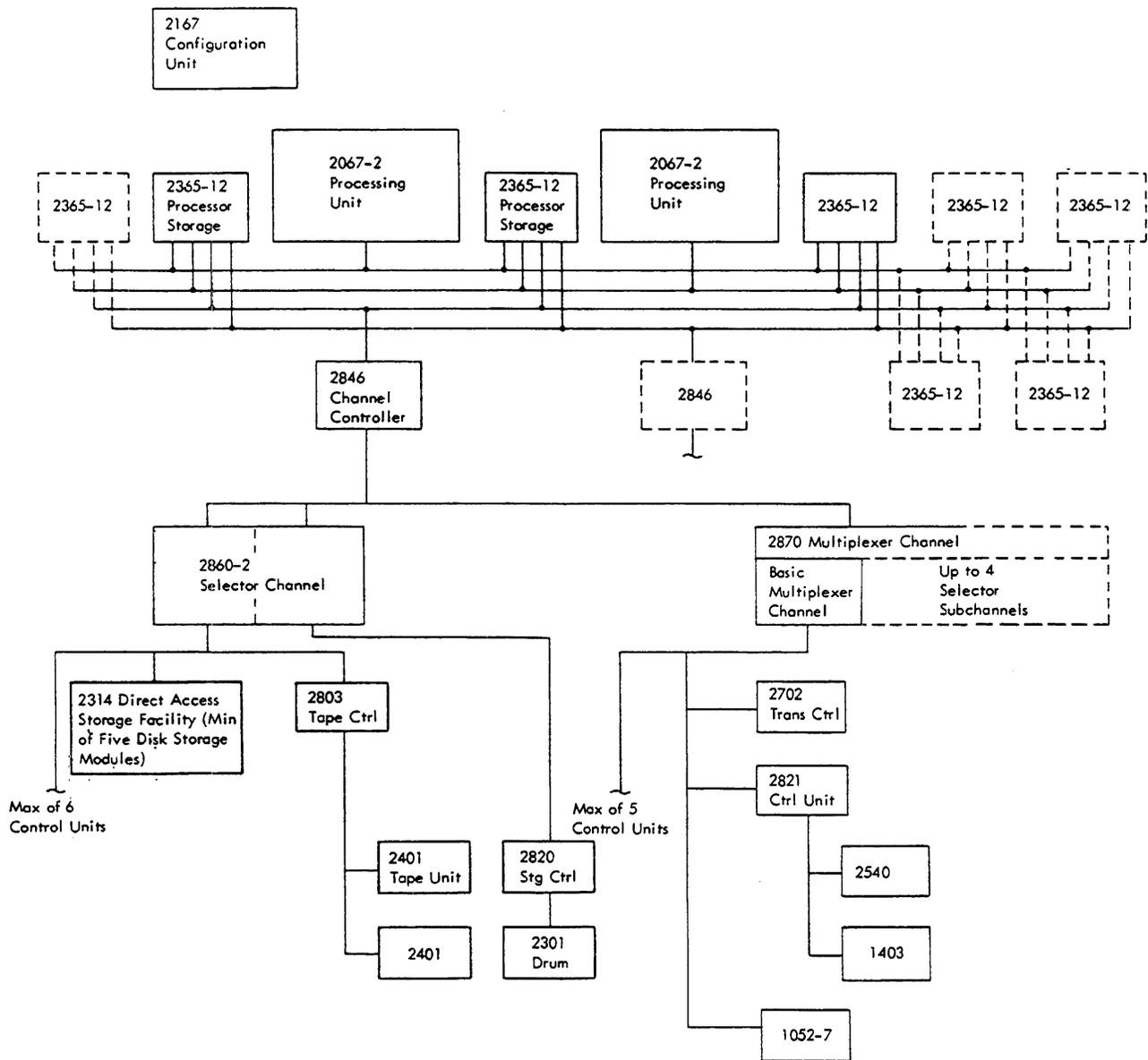
Figure 10. Model 67-2 Duplex System, Minimum Configuration
