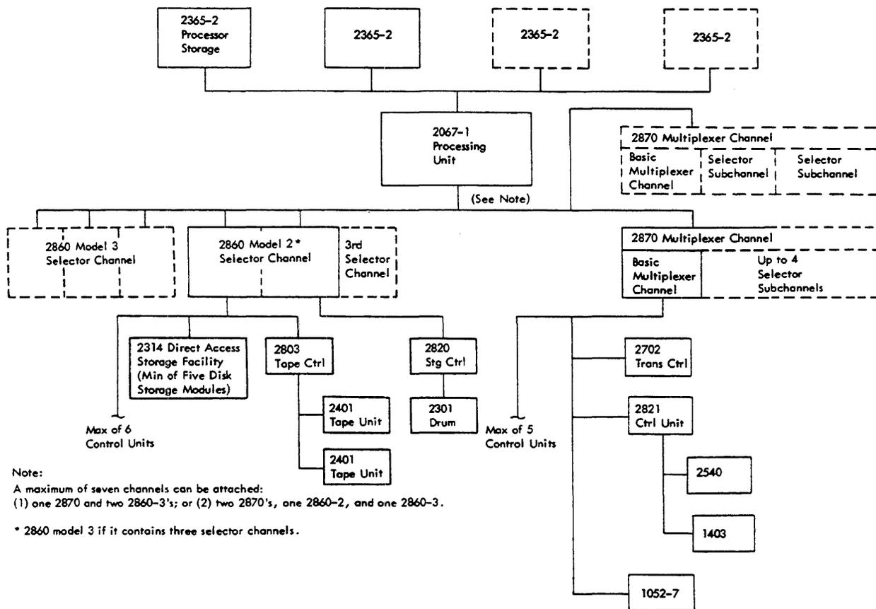
Figure 8. Model 67-1 Minimum Configuration
