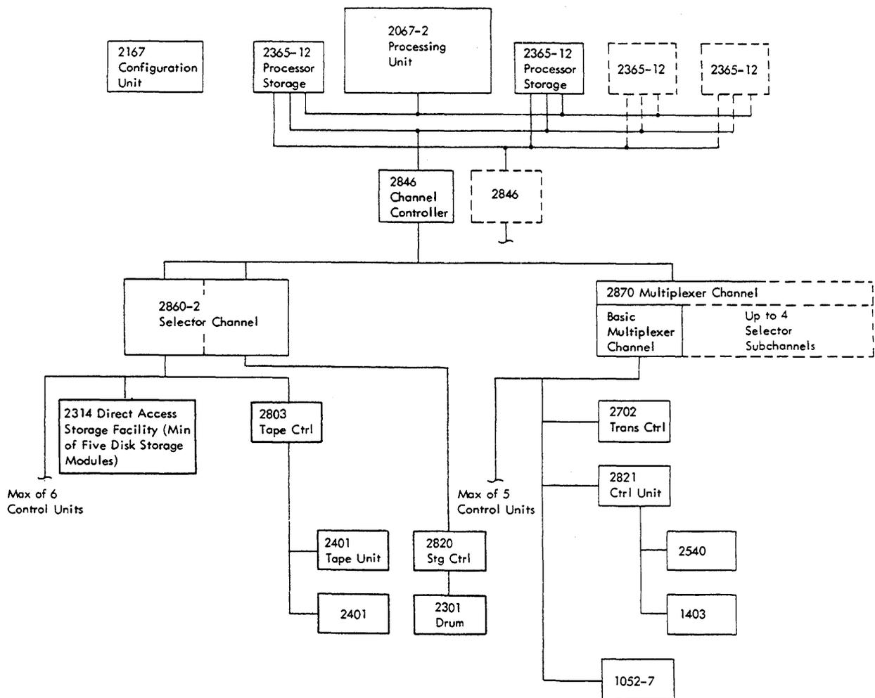
Figure 9. Model 67-2 Half-Duplex System, Minimum Configuration
