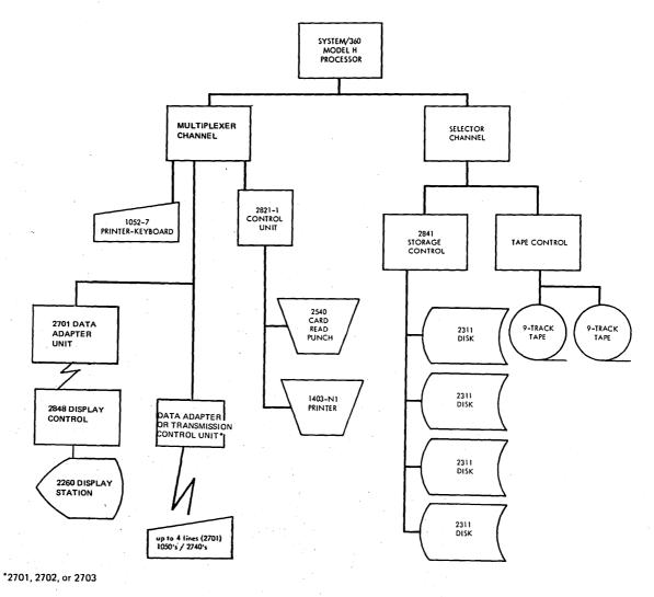
• Figure 14. Minimum configuration - Teleprocessing IMS/360
