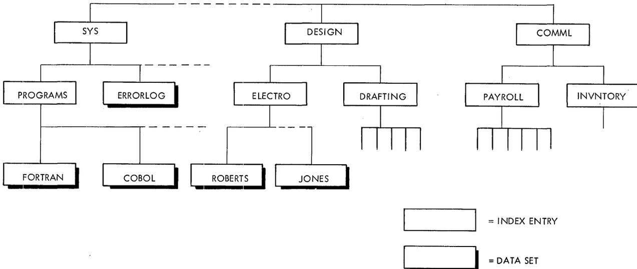
Figure 3. Simplified Diagram of a Catalog Organization
