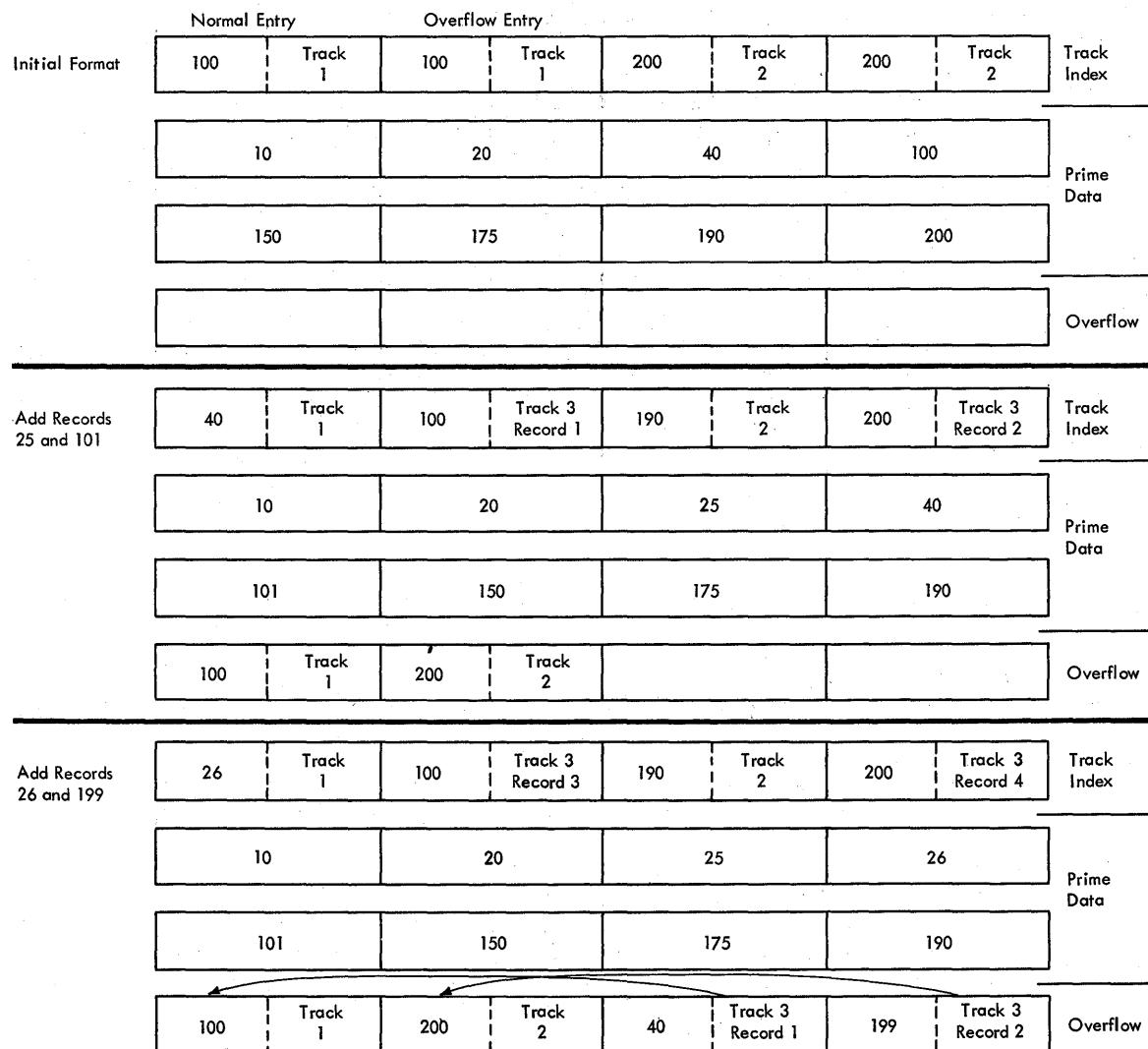
Figure 34. Adding Records to an Indexed Sequential Data Set
