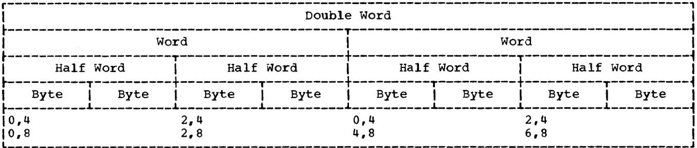
Figure 5-6. CNOP Alignment
