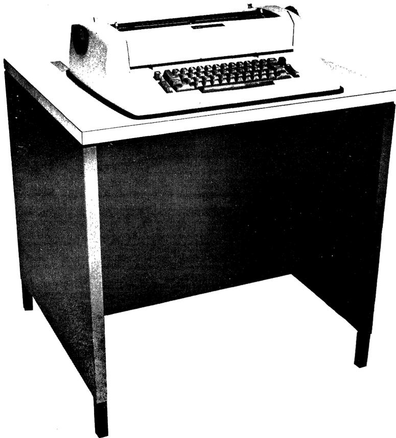
Figure 1. IBM 2741 Communications Terminal
