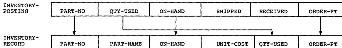
Figure 16. Movement of Data Resulting from Execution of MOVE CORRESPONDING.
