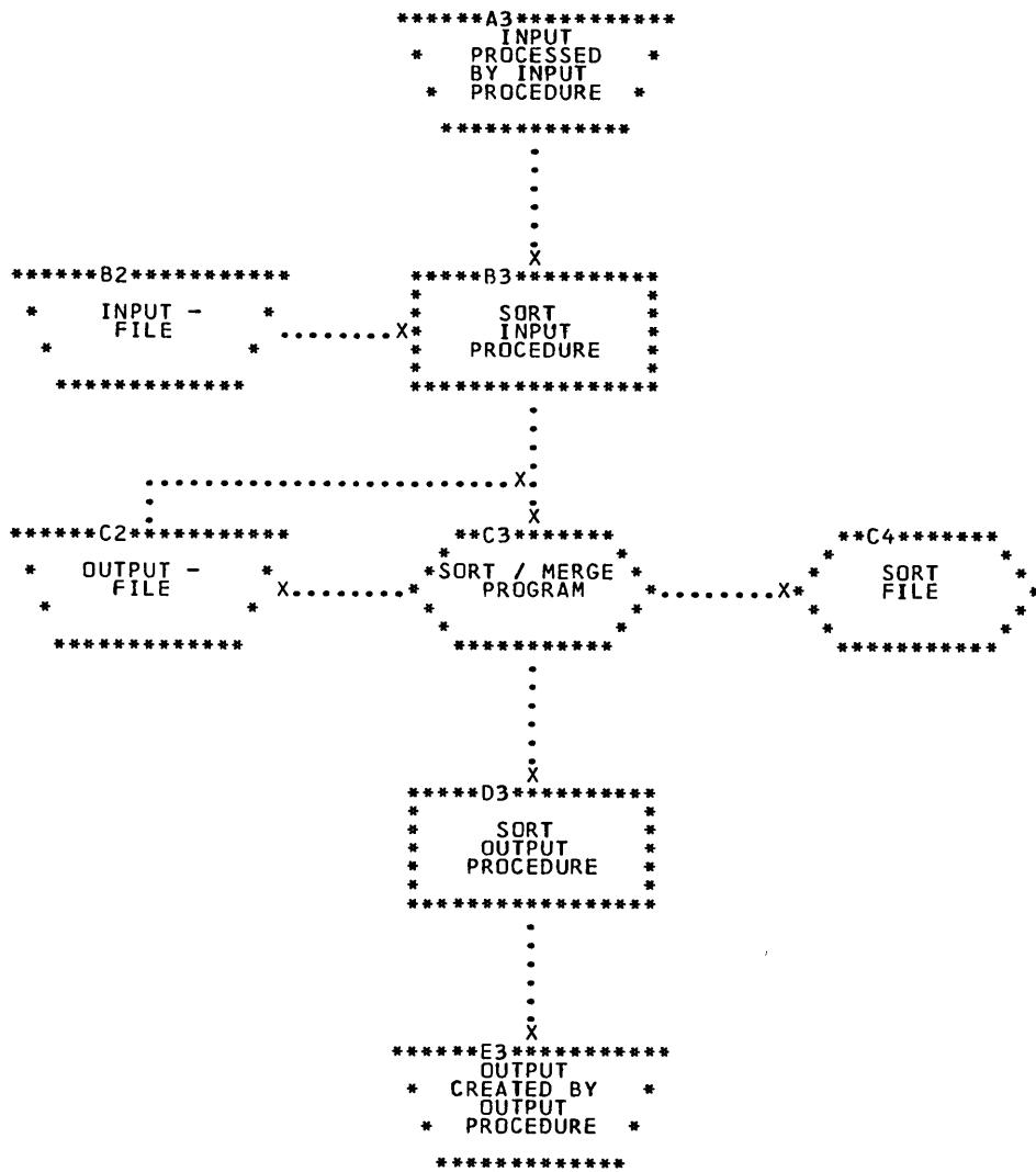
Figure S-1. Flow of Data through a Sort Operation.
