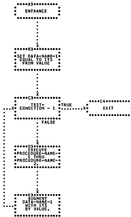
Figure 21. Logical Flow of Option 4 PERFORM Statement Varying One Data-name.
