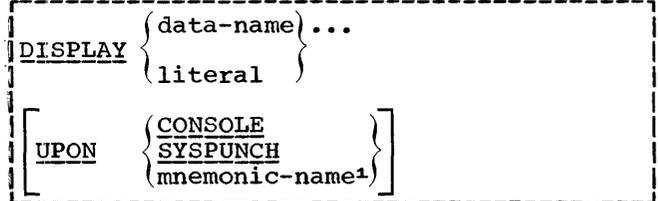
When the UPON option is omitted, the system logical output device (SYSOUT) is assumed. When UPON CONSOLE is written, the system console device is specified. When UPON SYSPUNCH is written, the system logical punch device is specified.
