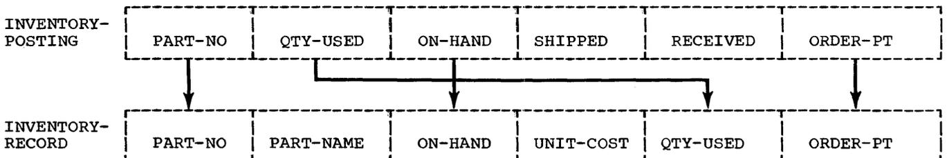
Figure 11. Data Movement Effected by MOVE CORRESPONDING Statement
