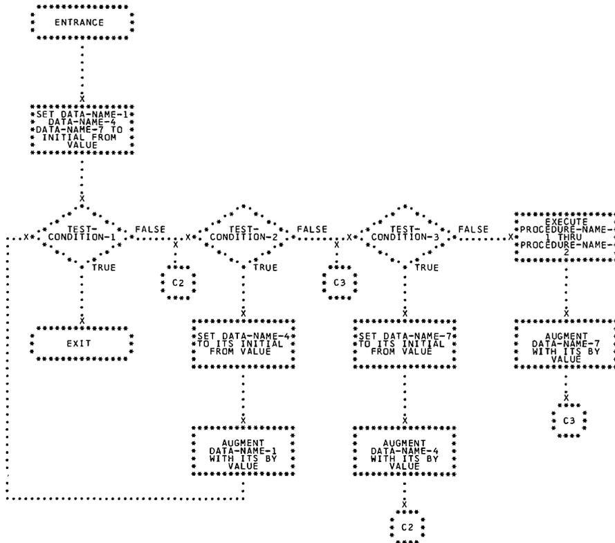
Figure 14. Logical Flow of Option 4 PERFORM Statement Varying Two Data-Names
