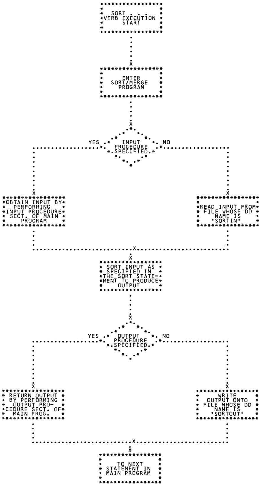
Figure 18. Flow of Data Through a Sorting Operation
