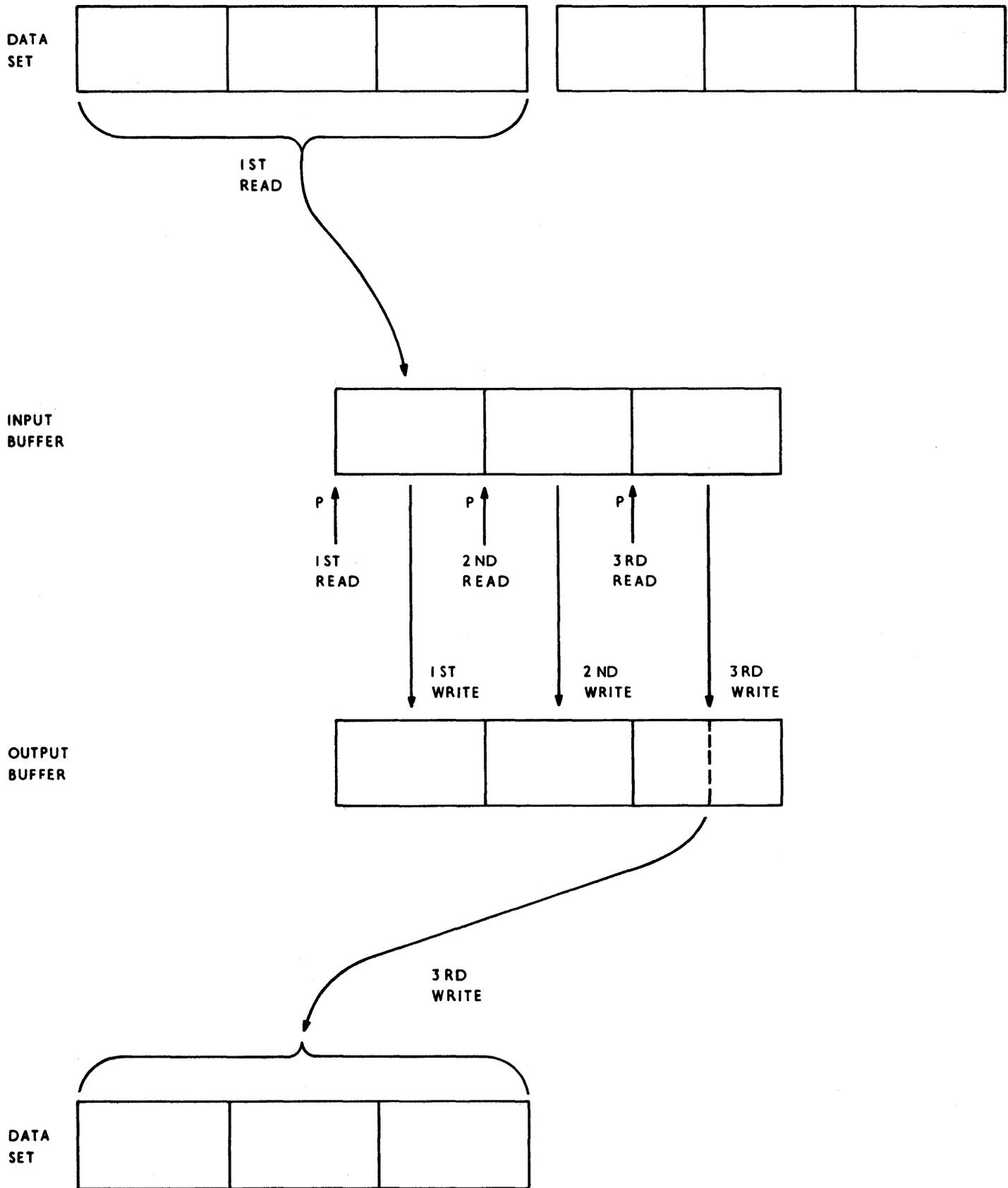
Figure 12.2. Locate mode input, move mode output
