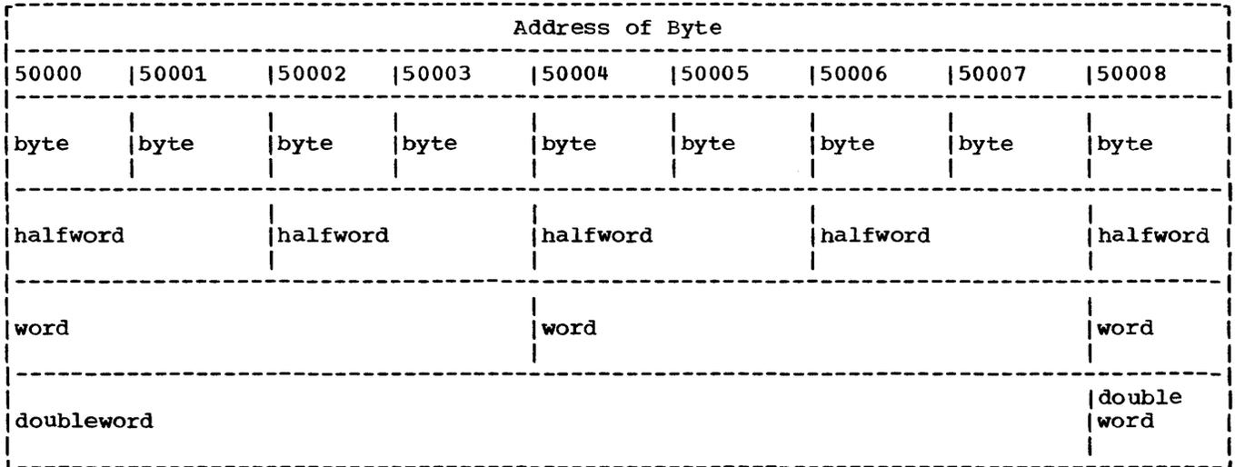
Figure 3.1. Section of main storage showing alignment of fixed length fields
