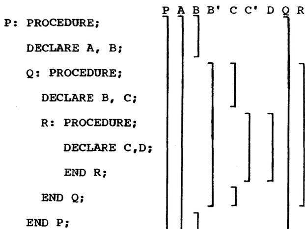
The lines to the right indicate the scope of the names. B and B' indicate the two distinct uses of the name B; C and C' indicate the two uses of the name C.
