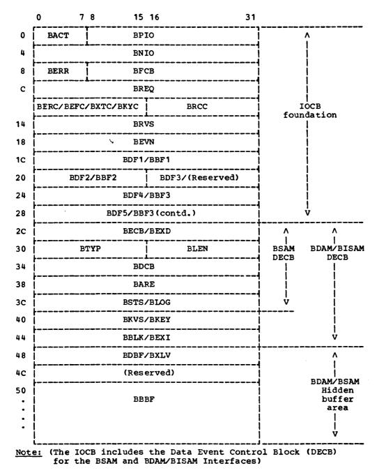
Figure 65. Format of the I/O Control Block (IOCB)
