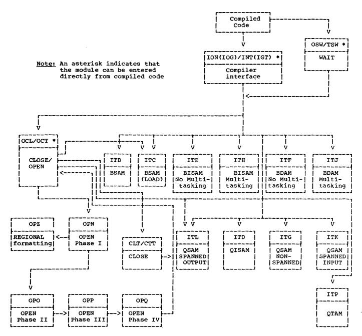
• Figure 15. Linkage of Access Modules in Record-Oriented I/O
