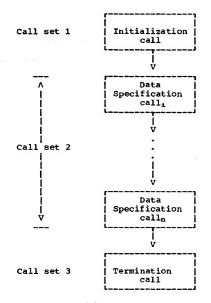
Figure 12. Object Program Structure of GET/PUT
