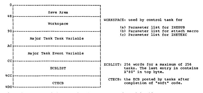
• Figure 76. Format of the Control Task Storage Area for Multitasking
