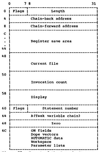
Figure 77. Format of the Dynamic Storage Area (DSA) for Multitasking
