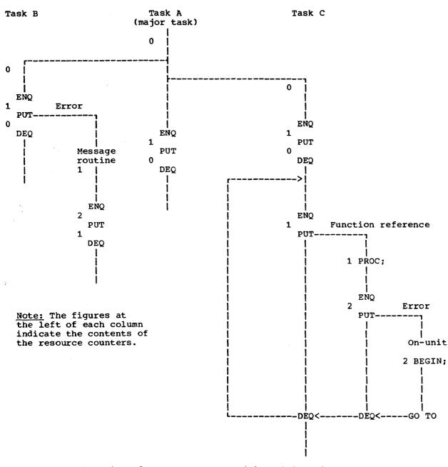
Figure 11. Allocation of SYSPRINT Resources in Multitasking
