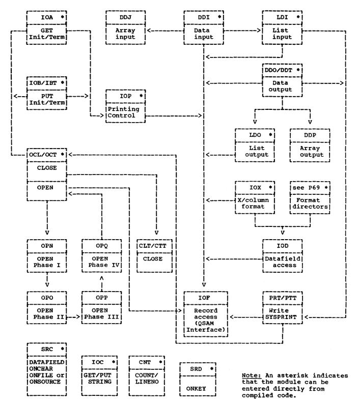
• Figure 9. Modular Linkage through Stream-Oriented I/O
