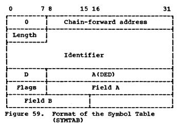
The symbol table consists of one or more entries which define the attributes, identifier, and storage location of variables which appear in the data list for data-directed I/O. Each SYMTAB entry contains the address of the next entry or a stopper.
