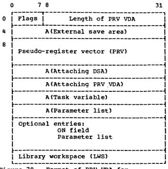
Figure 79. Format of PRV VDA for Multitasking
