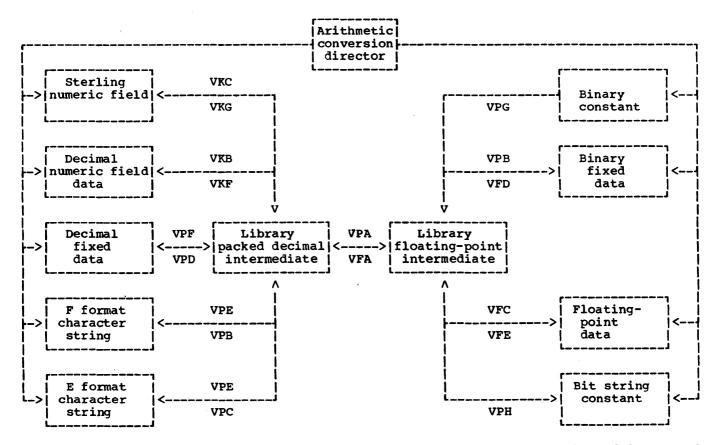
Note: The three-letter names, e.g., VKC, are the last three letters of the module name. A name above the flow lines indicates a conversion from left to right; a name below the line indicates a conversion from right to left.
