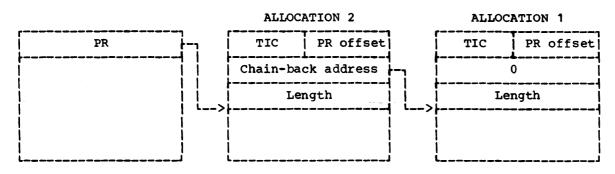
Figure 18. Storage Allocation for a Controlled Variable
