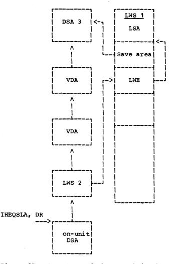
Figure 24. Structure of the DSA chain when the on-unit DSA is attached
