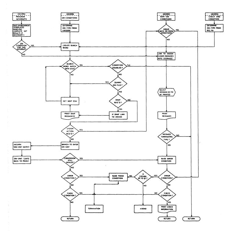
Figure 29. Flow through the Error Handling Routine (IHEERR)
