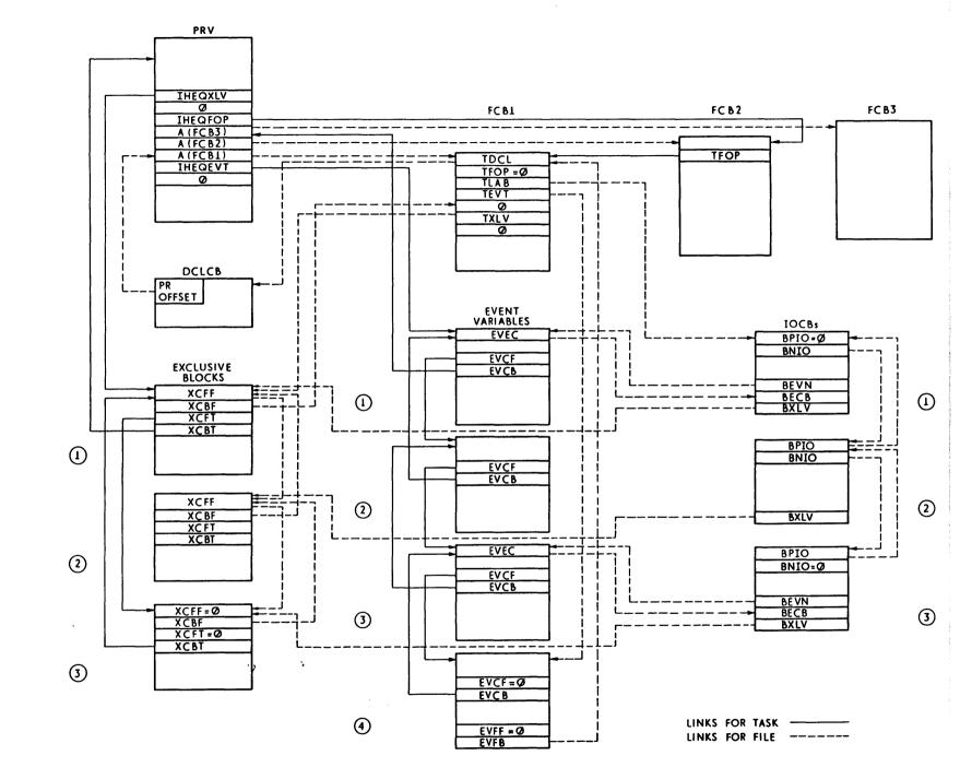
Figure 68. Example с, Chaining of I/O Control Blocks
