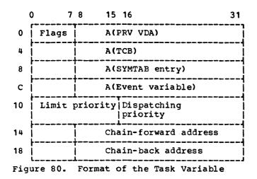
The task variable contains the task control information required by the PL/I Library. To enable subtasks to be detached when the attaching task is terminated, all task variables activated in a task are placed in a chain anchored in the DSA of the attaching task. Only the first two bits of the flag bytes are used:
