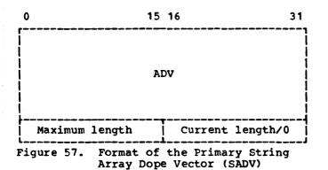
This control block contains information required to derive, directly or indirectly (through a secondary array of SDV entries), the address of elemental strings. The SADV is identical to the basic ADV, with the addition of a fullword which describes the string length.
