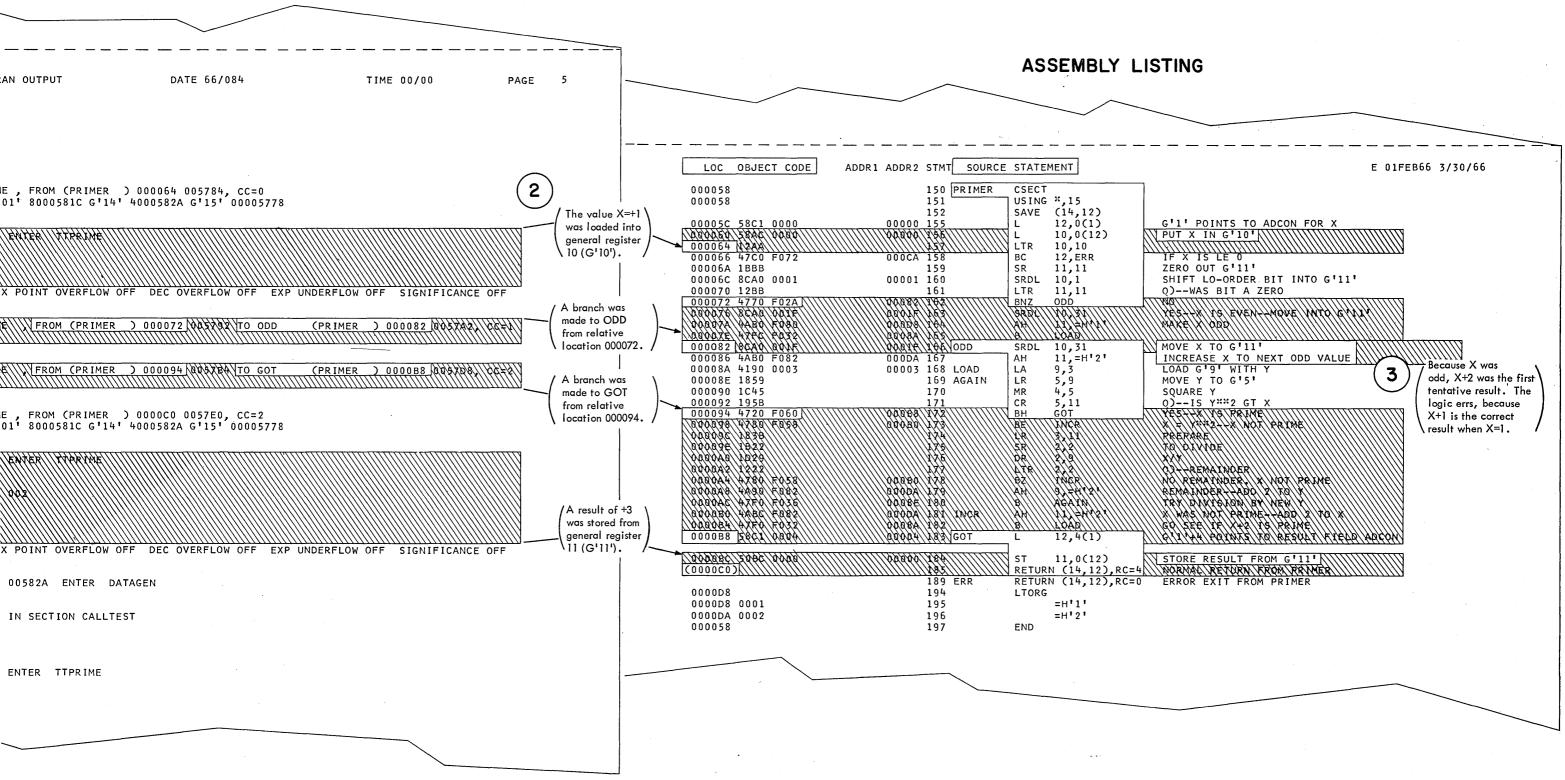
Figure 1. Use of TESTRAN to Detect an Error in a Program
