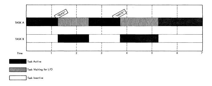
Time is shared between two tasks: Task A, a high-priority task, and Task B, a low-priority task. Task A controls the CPU whenever it is able to process data. The sharing of time is at irregular intervals, since it is governed by Task A's processing requirements.
