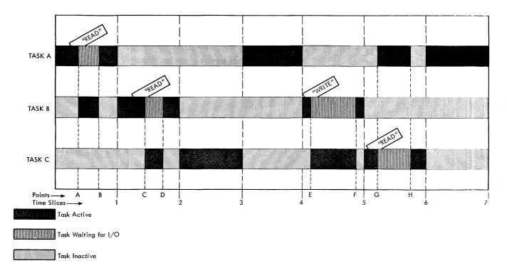
Time is divided, or sliced, in two distinct ways. If a task is unable to proceed, control is transferred to another task in essentially the same manner as in Figure 3 (i.e., on a <u>demand</u> basis). Time is also shared on a <u>scheduled</u> basis.
