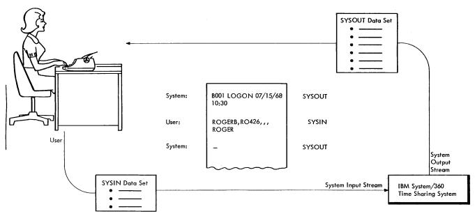
Figure 2. System Input and Output Streams
