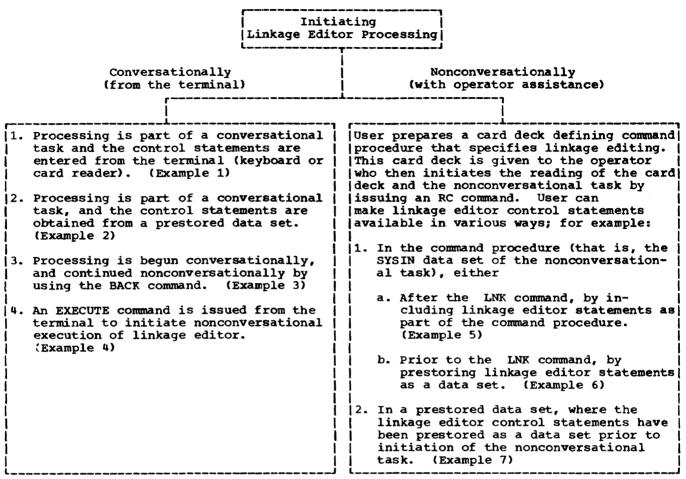
Figure 13. Methods for Specifying Linkage Editor Processing
