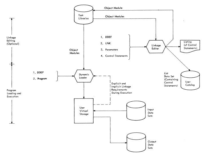
Figure 3. Object Module Combination in TSS/360
