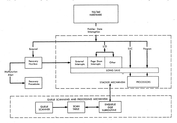
Figure 9. Interrupt stacker module overview
