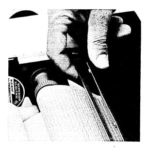
5. Cut the end of the new or remaining journal roll square, then fold the end at a 45° angle to form a point on the right side; slightly curl up the point.
