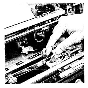
4. Place your fingers on both sides of the plastic handle of the ink roll assembly and your thumb on a flat surface near the top of the print unit. Carefully pull upward until the plastic fingers snap free of the mounting block. Then lift the ink roll assembly up and out of the printer.
