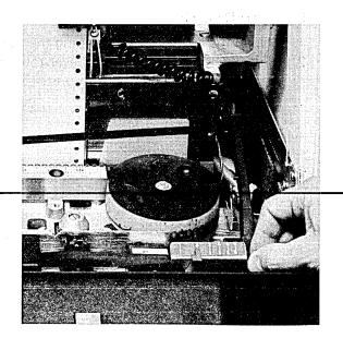
3. Pick up the print belt with the typeface up, and carefully place the belt around the pulleys and in back of the belt guard.
