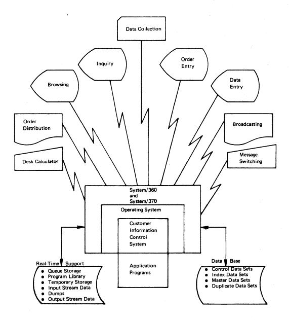
Figure 4. Data base/data communication system
