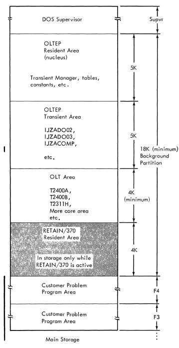
Figure 3-2. CLTEP Storage Allocation With RFTAIN/370 Active
