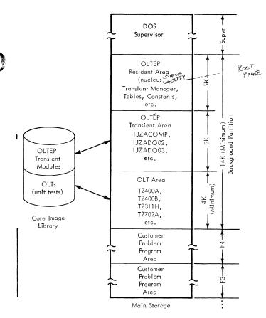
Figure 1-2. OLTEP Structure (Without RETAIN/370)
