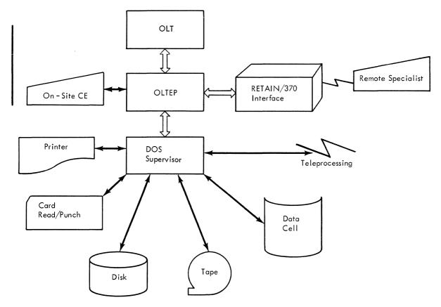
Figure 3-1 OLTEP System Relationship With RETAIN/370 Active
