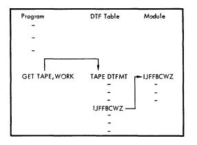
Figure 1-7 Relationship between program, DTF and logic module
