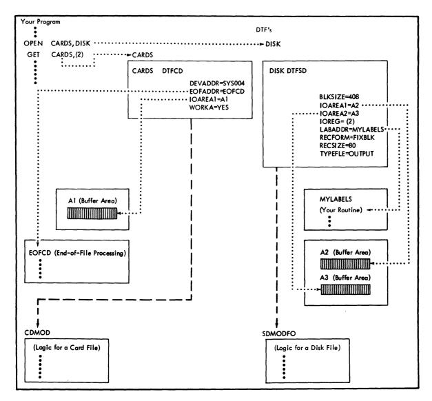
Figure B-1. Assembling Your Program DTFs and Modules Together (Example 1)
