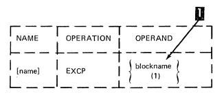
The EXCP (execute channel program) macro instruction requests physical IOCS to start an input/output operation for a particular I/O device. The blockname of the CCB established for the device is the only operand required in this instruction. 'Blockname' can be specified as a symbol or in register notation.
