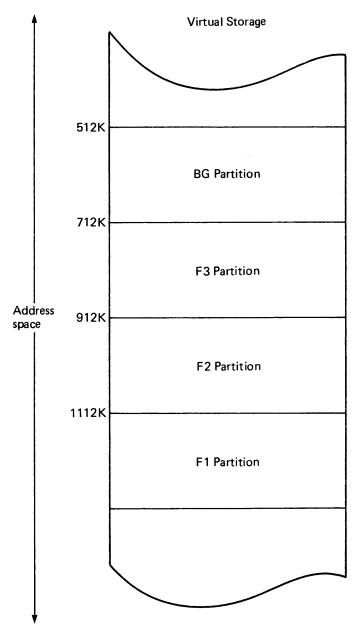
Figure 1-10. Partition Distribution in a Four-Partition System
