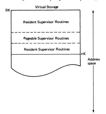
Figure 1-9. Supervisor Area in Virtual Storage Address Space
