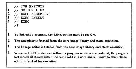
Figure 3-13. Job Control Statements to Assemble, Link-Edit, and Execute a Program in one Job
