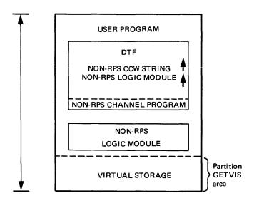
Figure 2-6. User Program Running in Virtual Storage without RPS Support
