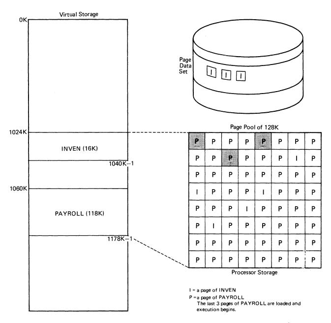
During execution, whenever a required instruction or some data is not present in processor storage, execution is interrupted by a so-called *page fault*. DOS/VSE must then read the required page into processor storage.
