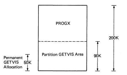
When PROGX is finished executing the partition GETVIS area size returns to its permanent allocation.
