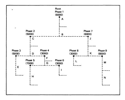
'The letters A through N represent control sections, which are organized to form nine phases in one program. The root phase resides in storage during the entire execution of the program. The remaining phases can overlay each other during execution.
