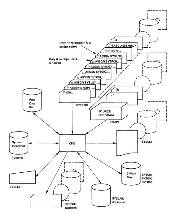
Figure 3-10. Device Assignments Required for an Assembly
