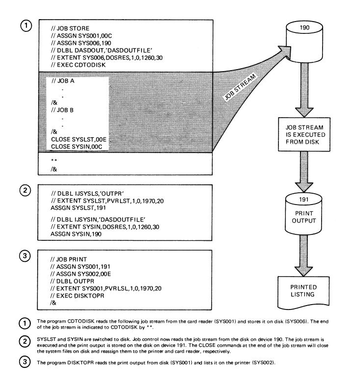
Figure 3-20. Processing System Input and Output Files on Disk
