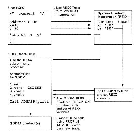
Figure 2. Data flow and trace facilities. Control and data flow are illustrated along with methods of tracing the values sent between REXX and GDDM.
