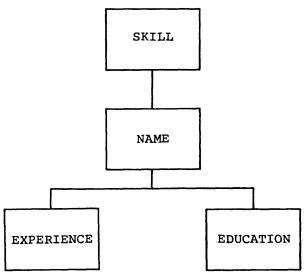
Figure 2-2. OS/VS Data Management -- IMS/VS Data Base Relationship
