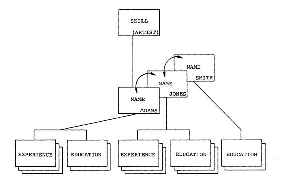
Figure 2-3. IMS/VS Data Base Record
