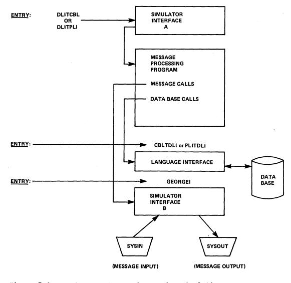
Figure 7-1. Message Processing Region Simulation
