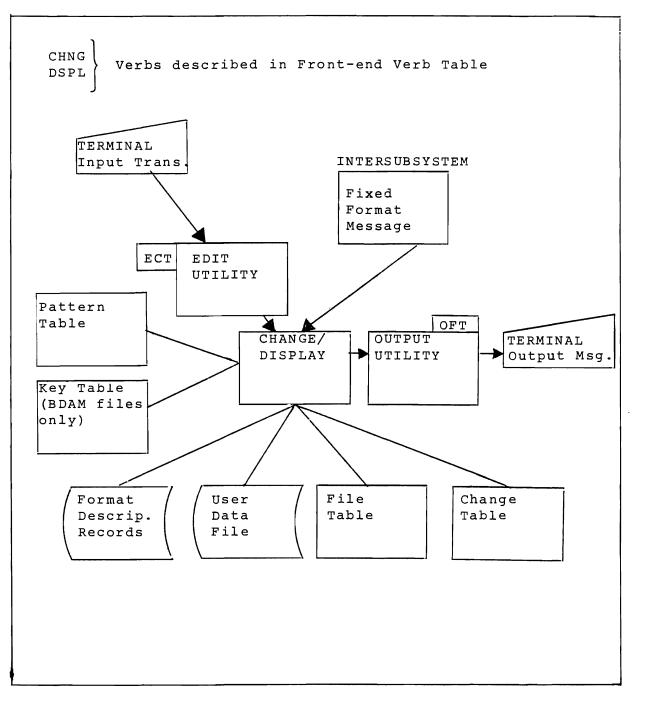
Figure 19. Functional Components of CHANGE/DISPLAY.
