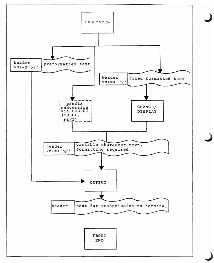
Figure 13. Format Options for messages to OUTPUT.
