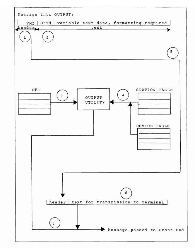
Figure 14. OUTPUT Processing Logic
