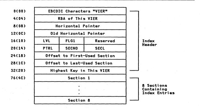
Figure 13. Format of the VTOC Index Entry Record (VIER)
