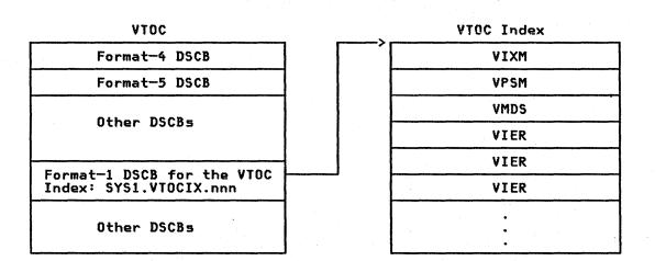
Figure 12. Relationship of a VTOC to Its Index
