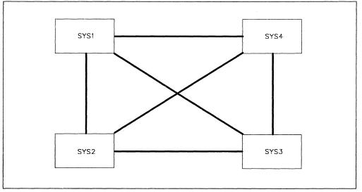
Figure 1-2. Fully-Connected Four-System Complex
