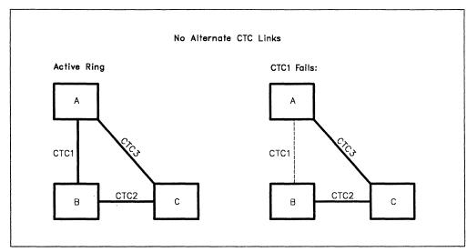
Figure 3-2. CTC Link Failure – No Alternate Available
