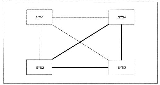
Figure 1-3. Three-System Ring – SYS1 Failed
