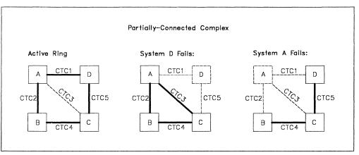
Figure 3-1. Recovery Problems with a Partially-Connected Complex
