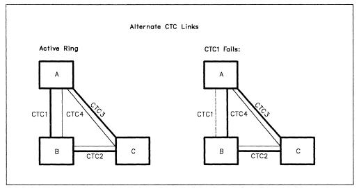
Figure 3-3. CTC Link Failure — Alternate Available
