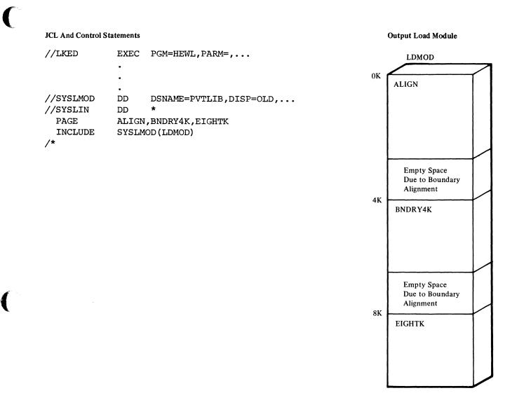
Figure 26. Output Load Module for PAGE Statement Example
