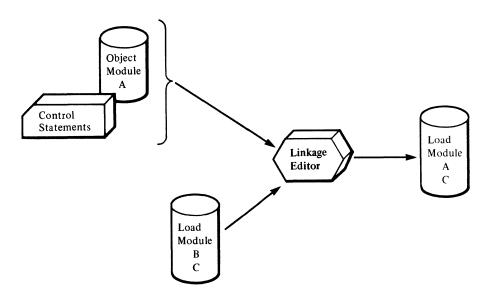
Figure 8. Linkage Editor Processing-Module Editing
