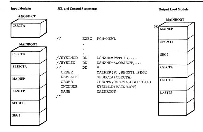
Figure 32. Ordering Control Sections
