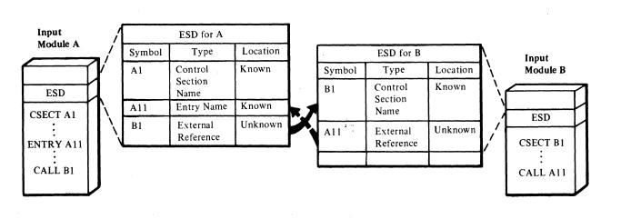
Figure 4. Use of the External Symbol Dictionary
