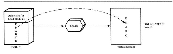
Figure 40. Loader Processing-Automatic Editing
