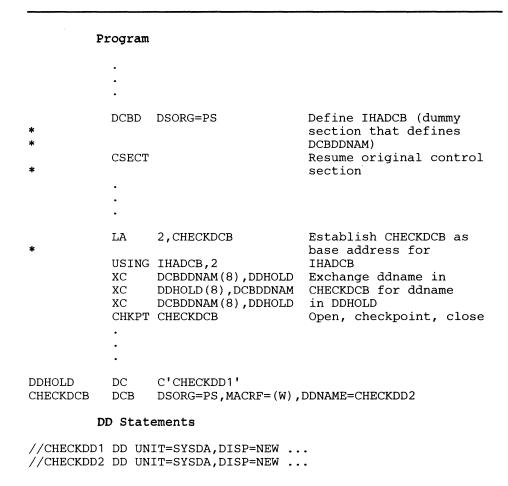
Figure 3. Using Two Sequential Checkpoint Data Sets to Ensure Restart
