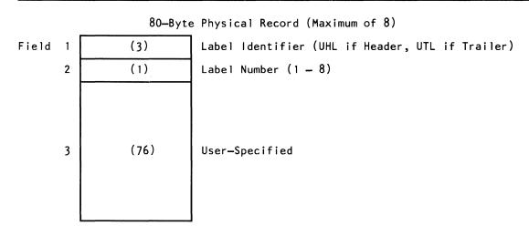
Figure 57. User Header and Trailer Labels
