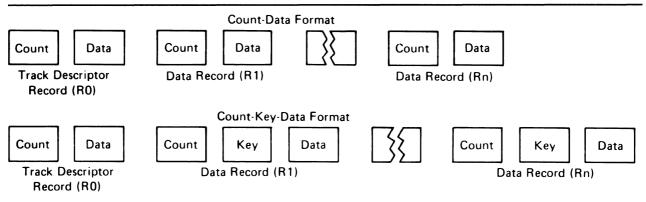
Figure 1. Direct Access Volume Track Formats
