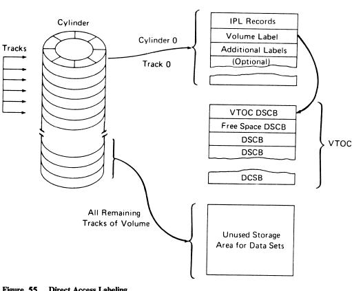
Figure 55. Direct Access Labeling
