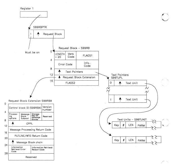
Figure 58. Structure of the SVC 99 Parameter List
