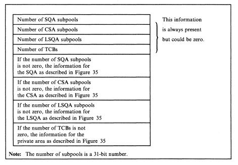
Figure 39. Allocated Storage Information for a Subpool List
