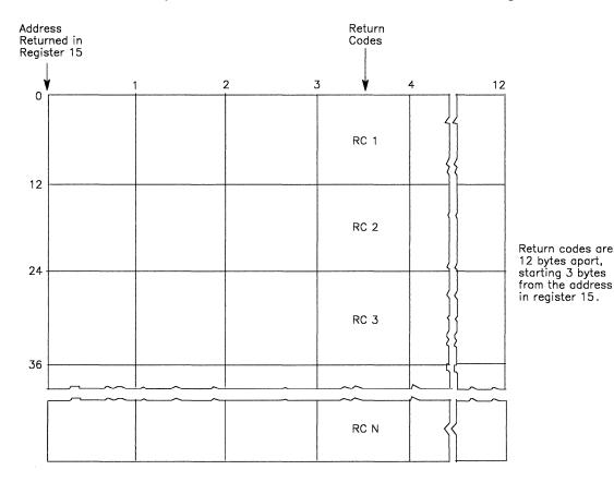
Figure 50. Return Code Area Used by DEQ
