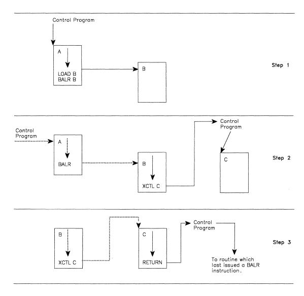
Figure 26. Misusing Control Program Facilities Causes Unpredictable Results
