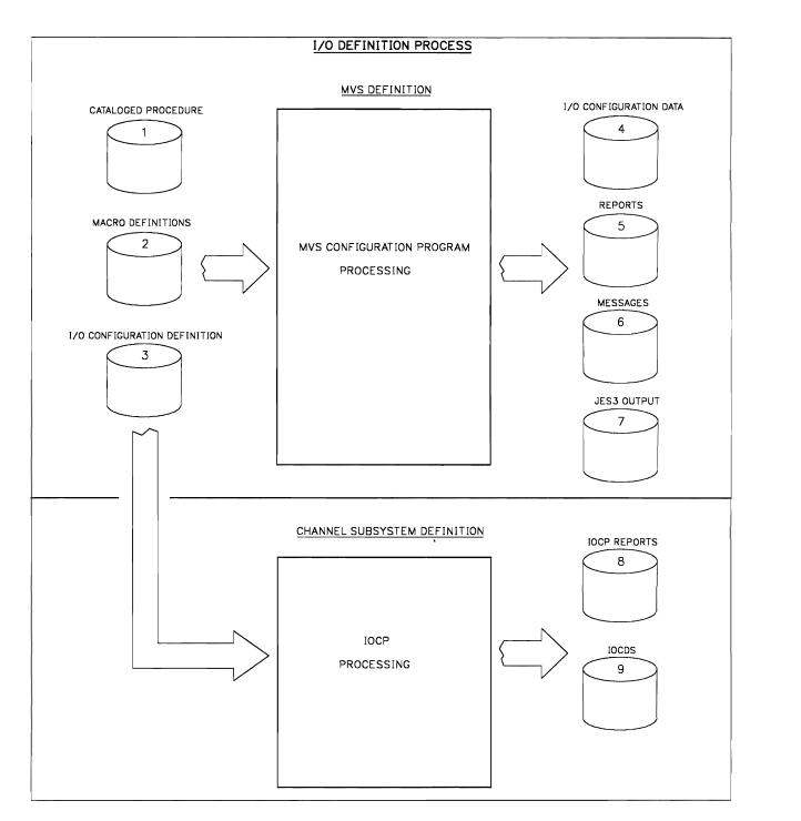
Figure 1-2. MVS and Channel Subsystem I/O Definition Process
