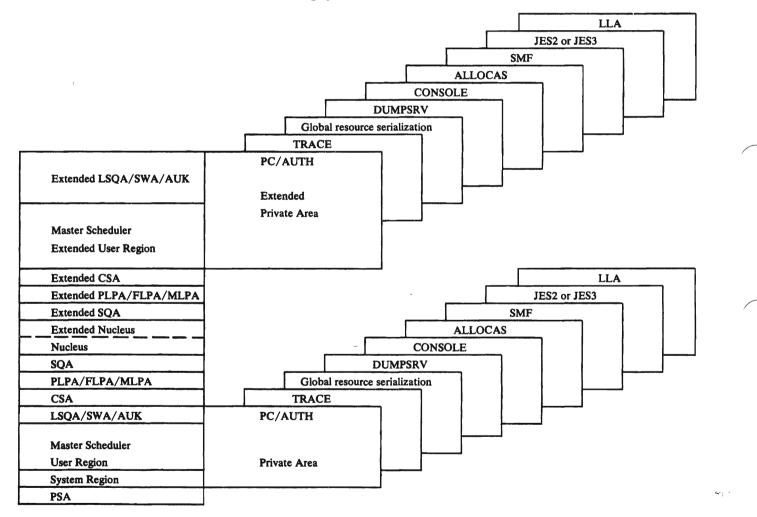
Figure 3-5. Virtual Storage Layout For Key MVS/XA Components.
