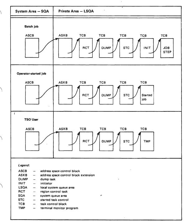
Figure 6-3. Address Space Task Control Block (TCB) Dispatching Queues
