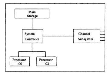
Figure 1-1. The 3081 Processor Complex
