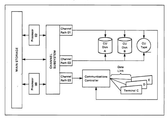
Figure 7-4. Multiple I/O Channel Paths
