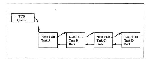
Figure 1-2. A Queue of Task Control Blocks
