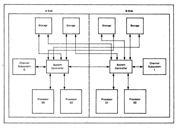
Figure 4-2. Tightly-Coupled Multiprocessing
