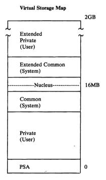
Figure 2-1. The MVS/XA Address Space
