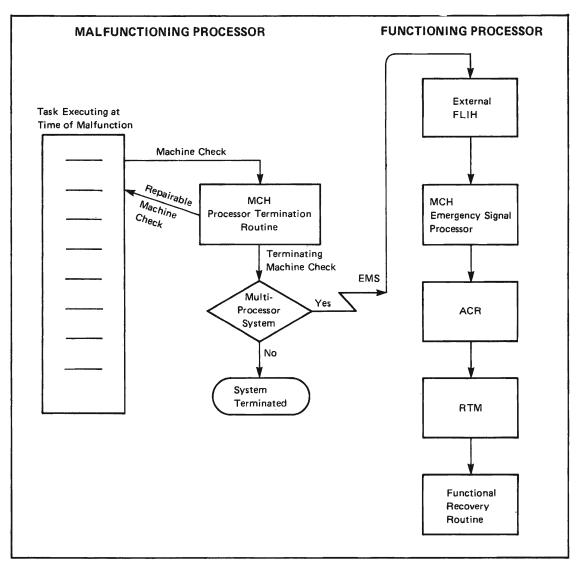
Figure 10-1 demonstrates the flow of control through the machine check handler and alternate CPU recovery.
