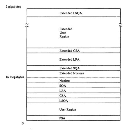
Figure 11-7. Virtual Storage at Exit from NIP
