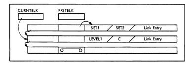
Figure 8 (Part 2 of 2). IGGOCLCB Example of Catalog Segment Block Handling
