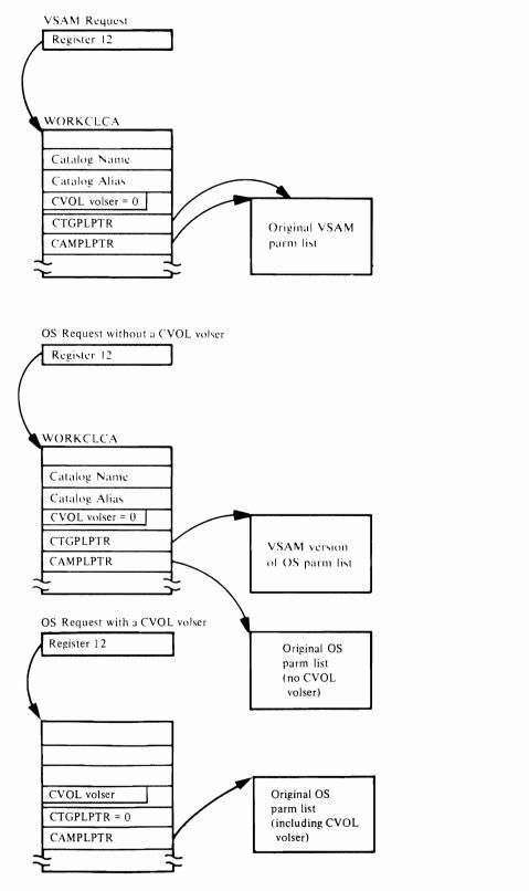
Figure 5. WORKCLCA at Processor Invocation
