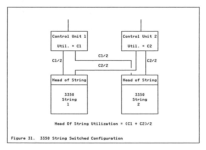
Consider the switched configuration in Figure 31. There a String 1 device ready to reconnect with Control Unit 1 faces two points of blockage: head of string and control unit. Even if String 1 is free, Control Unit 1 might by tied up serving String 2. In that case, reconnection could not occur; a full revolution (16.6 msecs) would be lost.
