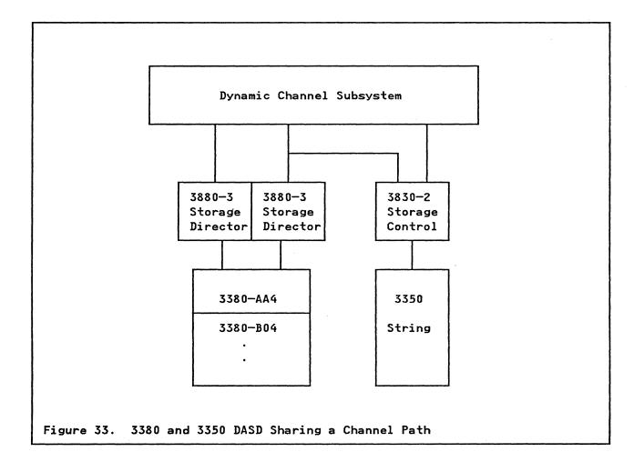
In such a case, any 3350 I/O requests initiated across the shared channel path may experience worse device response times than under MVS/370, because the the probability of a reconnection miss will become higher. Under MVS/370, the solution would be to disable the interface switch to the 3350 string on the shared path. However, in the event of a path malfunction, this would require operator intervention to enable the 'availability' path.
