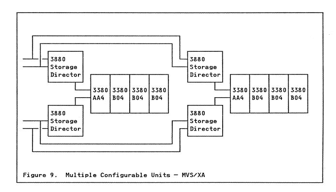
In an MVS/370 environment, this configuration would only be valid when attached to a multiprocessor or dyadic system with two Channel Sets configured. For normal operation many installations would VARY OFF two of the four channel paths because of the negative effect the additional level of DASD switching has on performance. In the event of a component failure, operator recovery action would be required to enable the alternate 'availability' paths.
