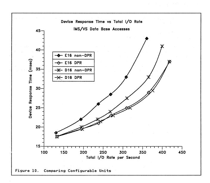
The actual sizing of a Configurable Unit is related to the type of workload for which it will be used. For each environment a balance has to be found between the number of channel paths, control units, and devices, while retaining all of the availability requirements.
