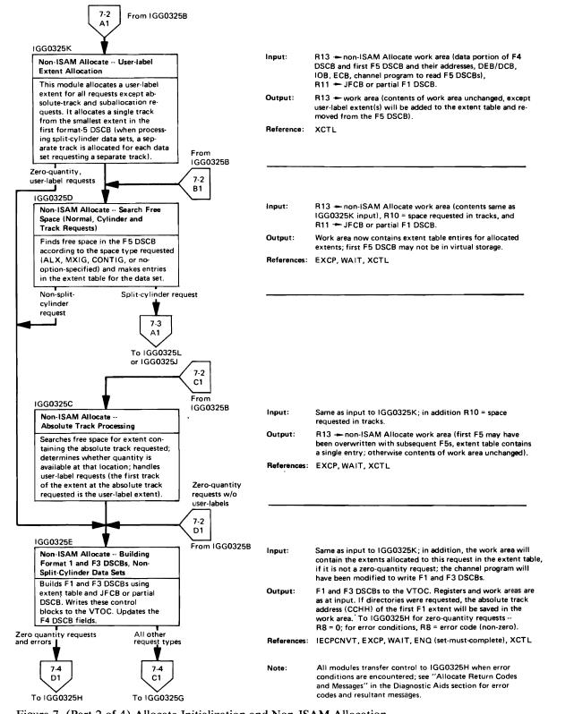
Figure 7. (Part 2 of 4) Allocate Initialization and Non-ISAM Allocation
