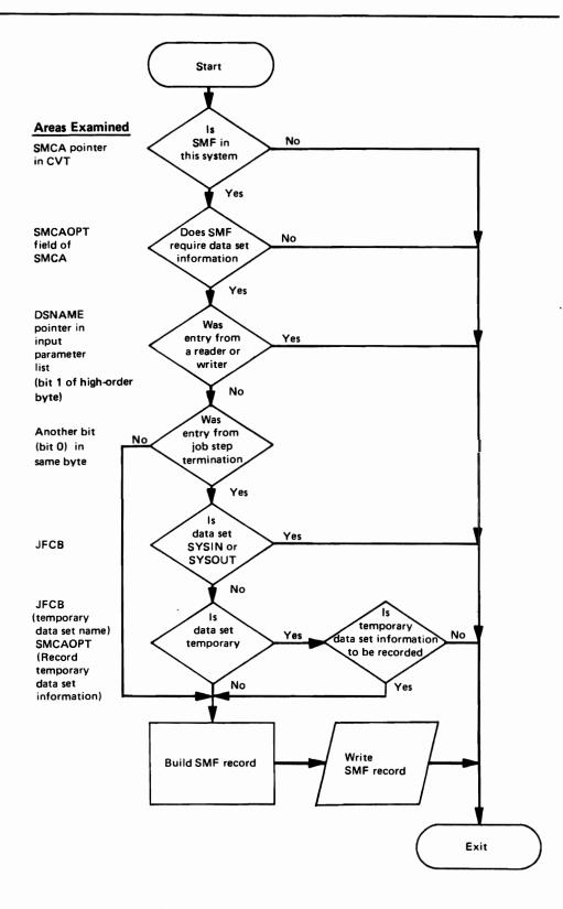
Figure 4. Logic used to determine whether SMF records are needed (scratch routine)
