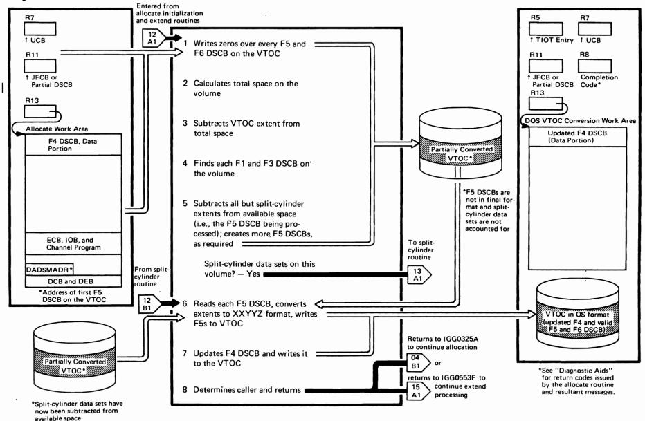
© Diagram 12. DOS VTOC Conversion—Initialization, Non-split Cylinder Data Set Conversion and Termination
