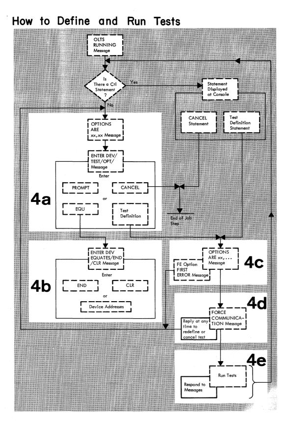
Figure 9. How To Define and Run Tests
