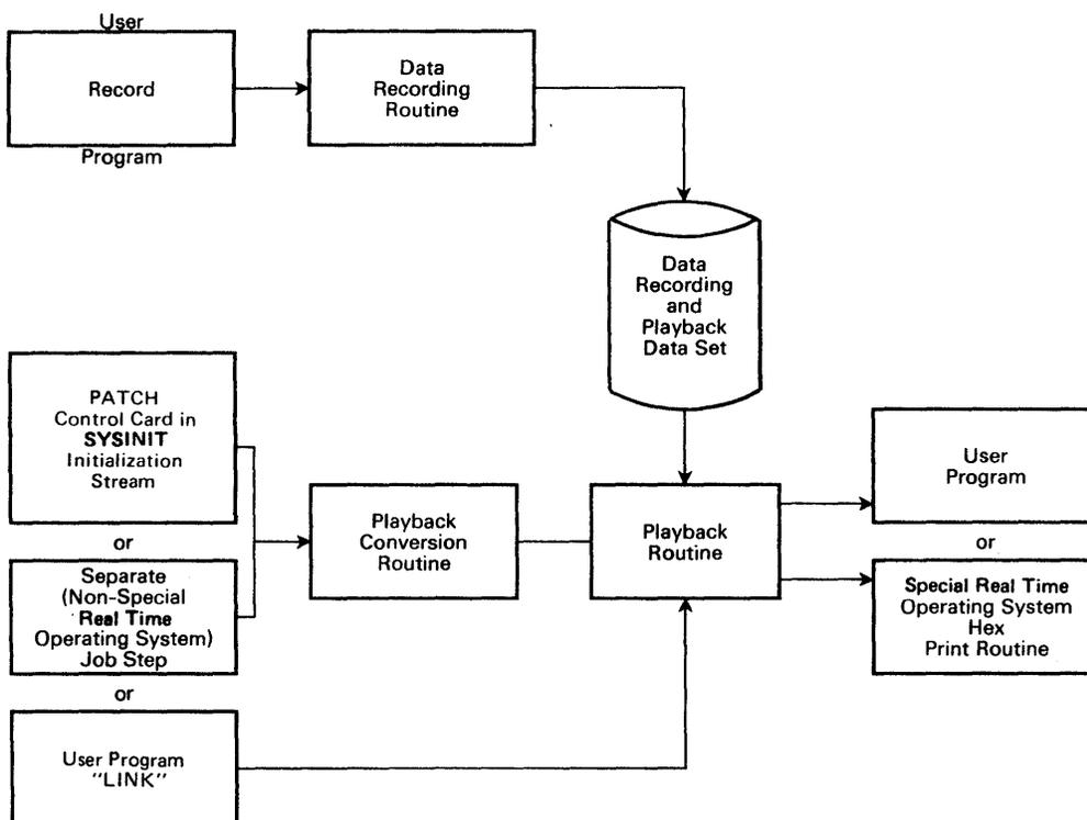
Figure 2-11. Data recording and Playback Processing Overview
