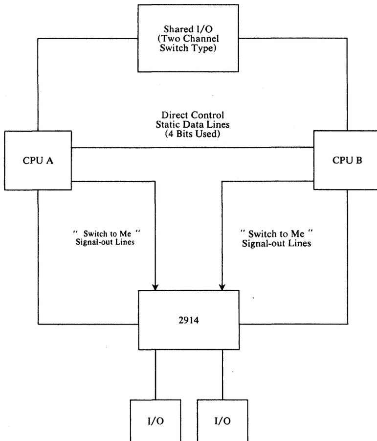
Figure 2-30. System With Automatic 2914 Switch
