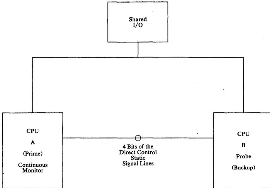
Figure 2-28. Probe Function Failure/Restart Feature
