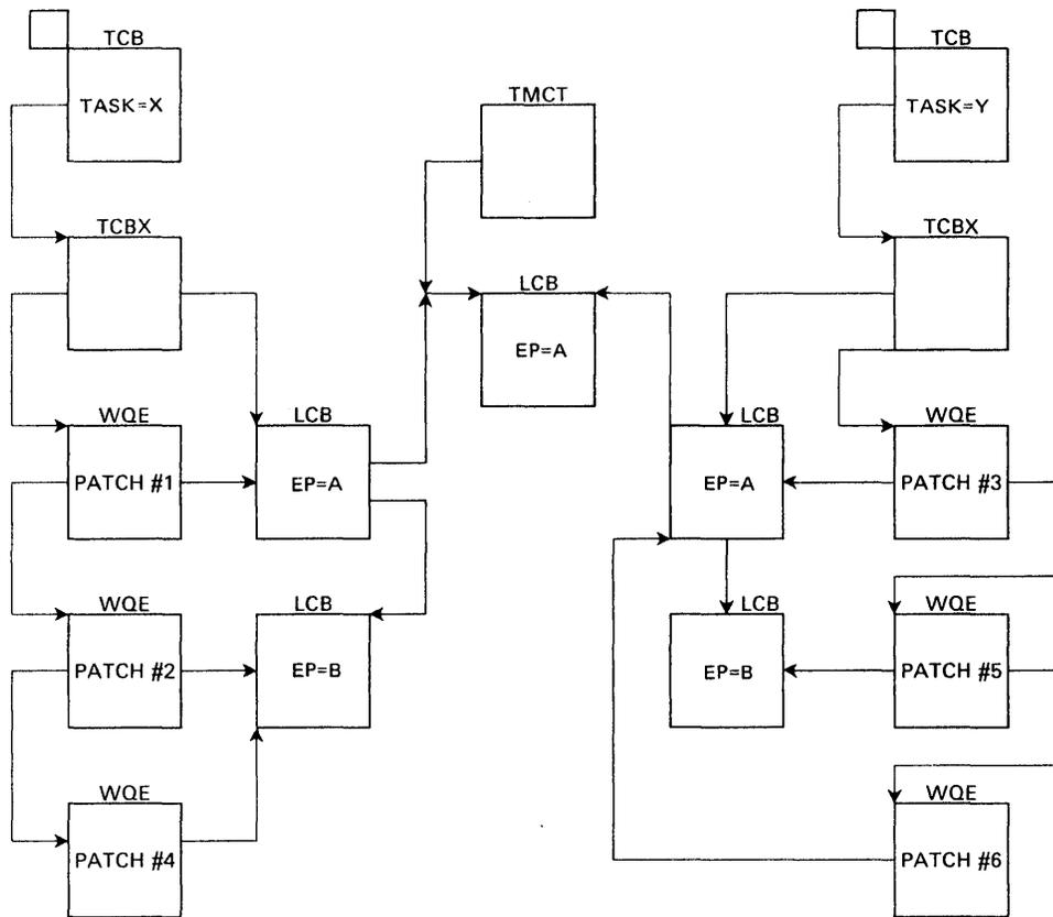
Figure 2-5. Control Blocks Built for Example 1
