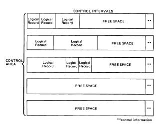
Figure 10. Distributing Free Space in a Key-Sequenced File
