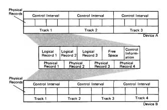
Figure 9. Control Intervals, Physical/Logical Records, and Tracks
