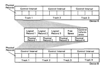
Figure 9. Control Intervals, Physical/Logical Records, and Tracks
