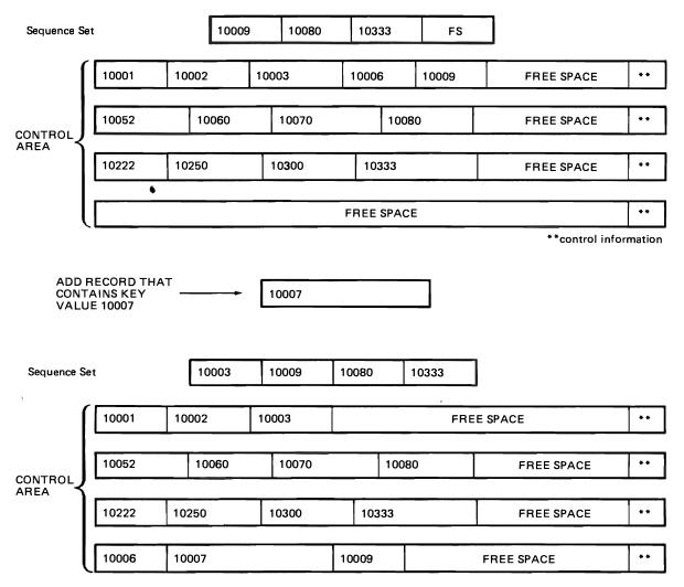
Figure 17. Control Interval Split
