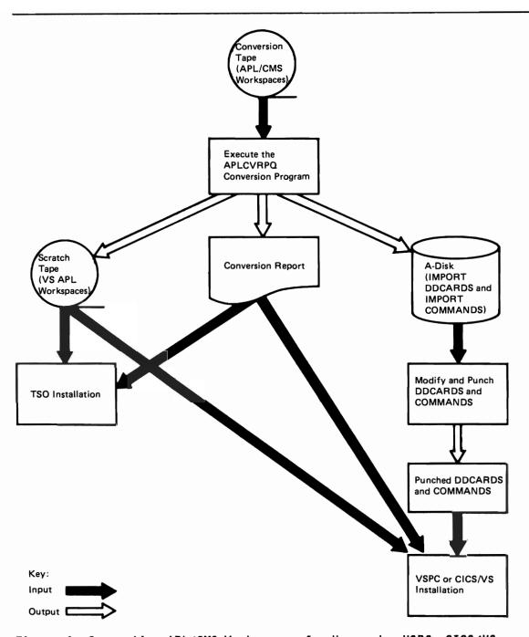
Figure 6. Converting APL/CMS Workspaces for Use under VSPC, CICS/VS, or TSO
