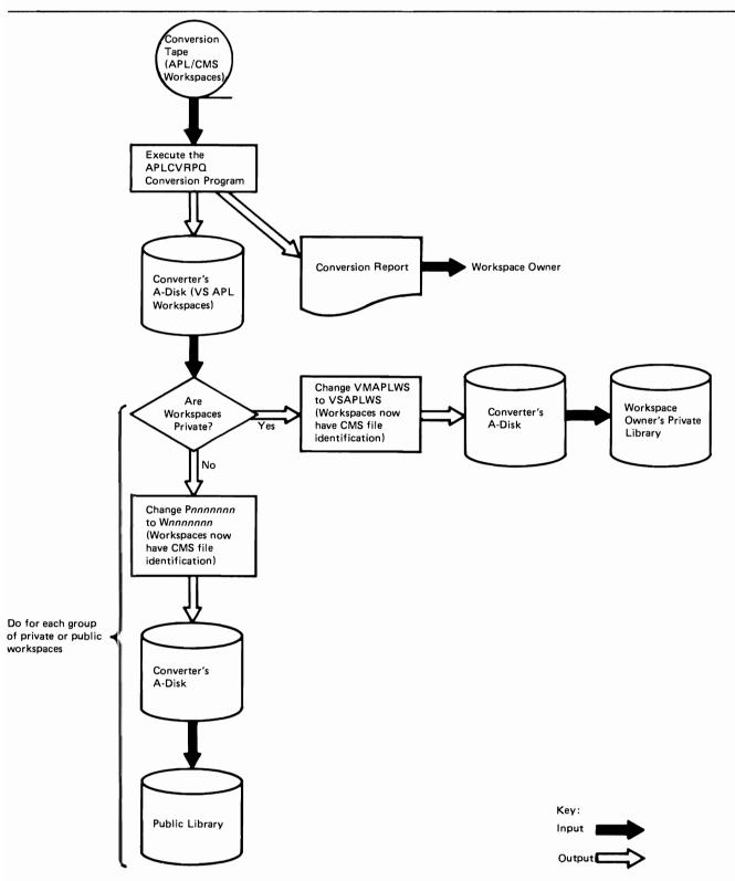
Figure 5. Converting APL/CMS Workspaces for Use under CMS
