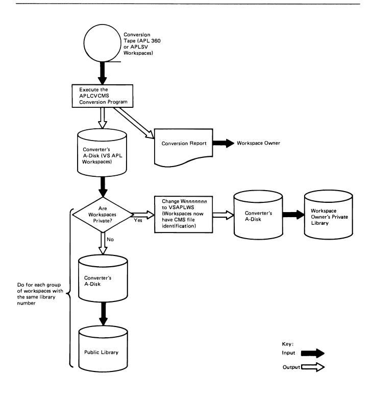
Figure 7. Converting APLSV or APLN360 Workspaces for Use under CMS
