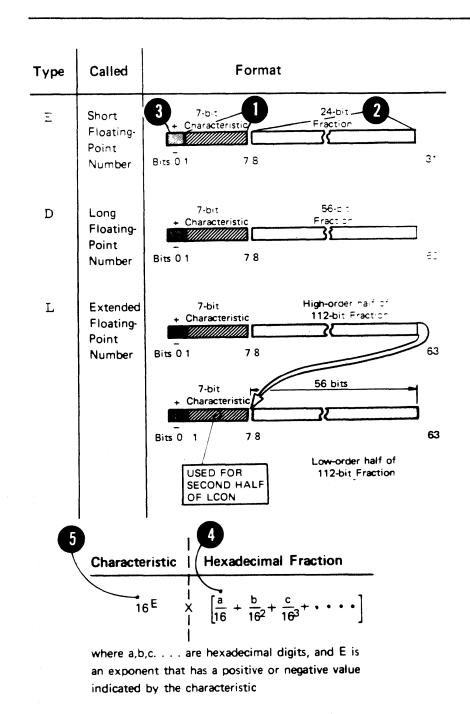
Figure 32. Floating-Point External Formats
