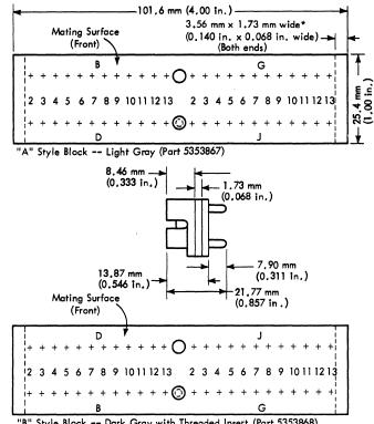
"B" Style Block -- Dark Gray with Threaded Insert (Part 5353868) "B-" Style Block -- Dark Gray, No Threaded Insert (Part 5353869)
