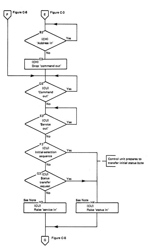
*Note:* The byte on 'bus in' must be valid within 100 ns after the raising of the in tag.
