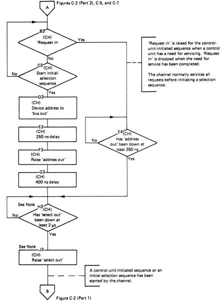
Note: All mention of 'select out' assumes proper operation of 'hold out' as well. Therefore, 'select out' up means 'select out' and 'hold out' are up, and 'select out' down means either 'select out' or 'hold out' is down.
