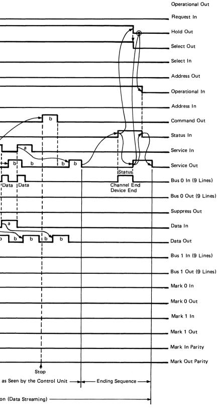
Figure C-13. Data-Streaming Operation on Block-Multiplexer Channel
