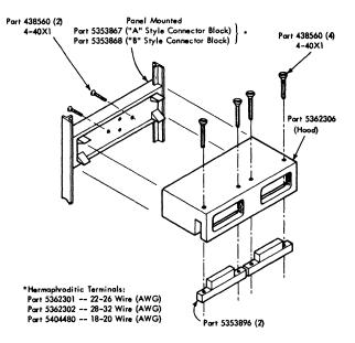
Figure B-2. Panel Mount with Optional Strain Relief
