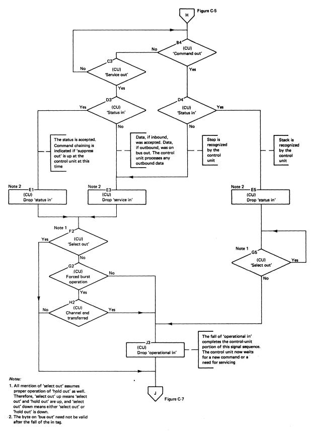
Figure C-6. Response to Stack/Stop/Accept
