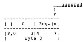
The contents of the accumulator are stored into the SVP storage. The 16bit storage address is obtained from an adjacent pair (even+odd numbered) of LS registers. The even numbered LS register, containing the high order byte of the storage address, is defined by instruction bits 4,5 and 6. Instruction bit 7 is ignored. The contents of LSZR define the LS-zone. The storage address (in the LS-reg. pair) is automatically incremented by 1 via the ALU.
