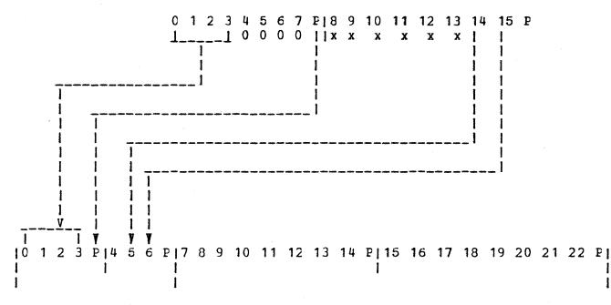
Note: ALU bits 4....7 must be zero to ensure correct parity for the key. ALU bits 8....13 are ignored.
