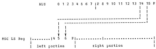
Bit 16=1, means store operation to key storage. In this case ALU bits 8....14 are stored, as shown. ALU bits 8...11 represent the key, while the rest of the bits have the following functions:
