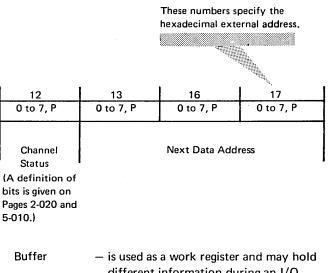
different information during an I/O operation. Its main use is to hold one I/O data byte for preparing halfword transfers to main storage with read operations.
