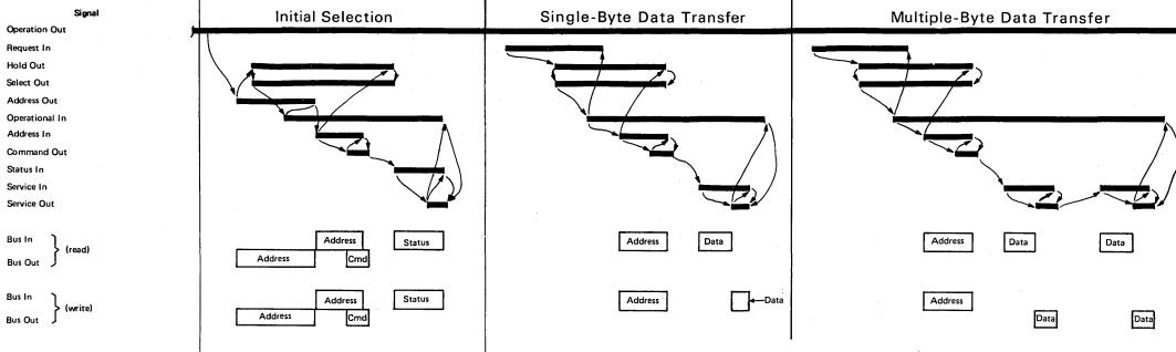
The microprogram controls the activation and inactivation of the necessary tag out lines in proper sequence. The address control unit in turn answers, by activating and inactivating the appropriate tag in lines.
