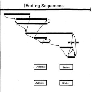
With channel end alone, or channel end with device end, the status byte is set into the unit status byte in the UCW. STI is followed by SVO, indicating that the status is accepted. Subsequently the 'interrupt request' FL is set. which in turn causes activation of the 'interrupt request' line to the IPU. Device end alone is always stacked until an interrupt occurs or a 'TIO' instruction is issued. Device end status is then fetched from the control unit.
