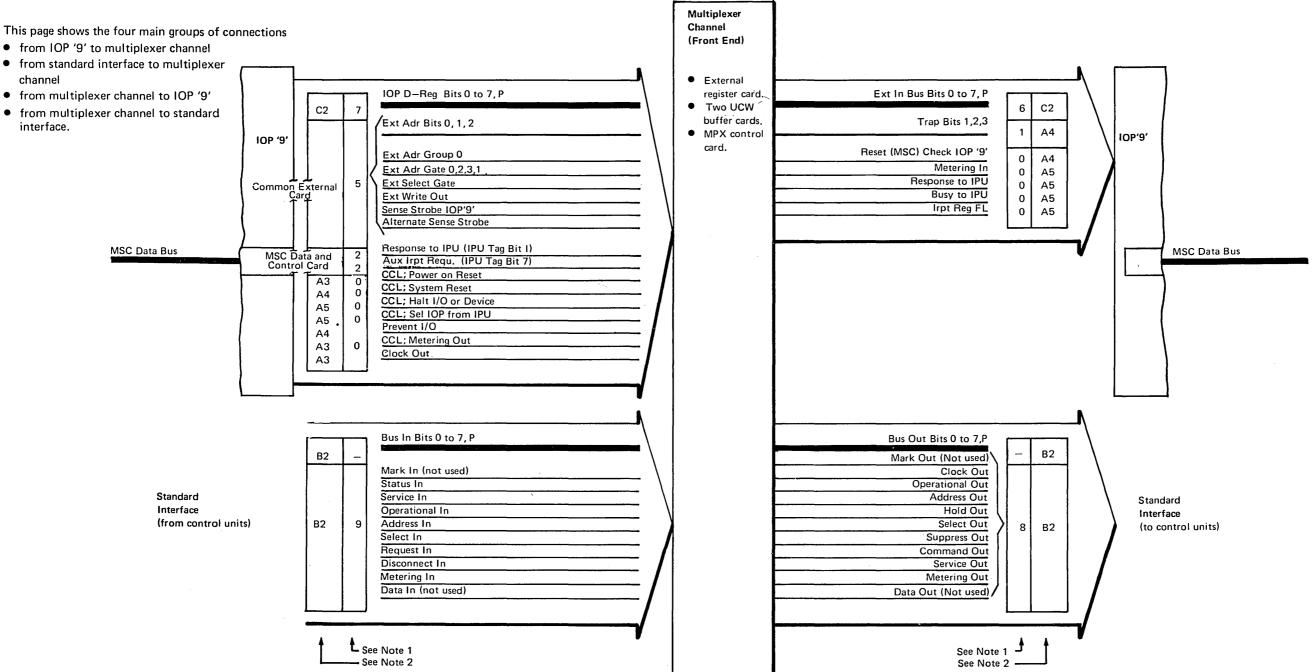
Note 1: The numbers in these columns define the line groups as they are shown on Page 4-010 and described on Pages 4-030 and 4-040. Note 2: These letter/number combinations define the plug locations of the cables on multiplexer channel board.
