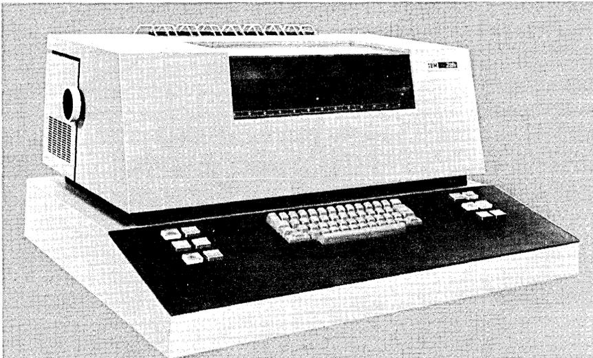
Figure 3. IBM 3215 Console Printer-Keyboard
