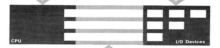
Specialized integrated adapters, integrated attachments, a direct disk attachment, and a standardized channel are used for attaching I/O devices. The integrated adapters, attachments, and the channel work like System/360 channels. For programming purposes, the I/O attachment facilities are considered to consist of three channels.
