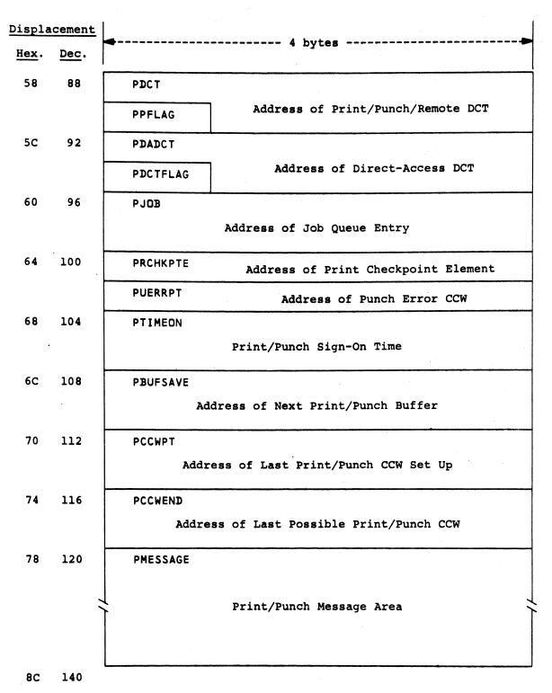
Figure 4.3.1 -- OUTPUT SERVICE PCE WORK AREA FORMAT
