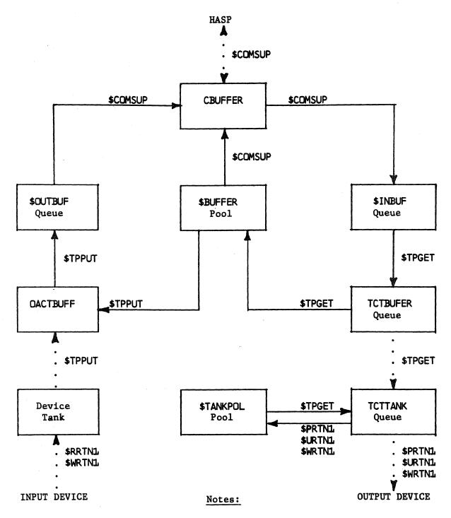
Solid lines indicate buffer or decompression tank flow with or without data. Broken lines indicate data flow only.
