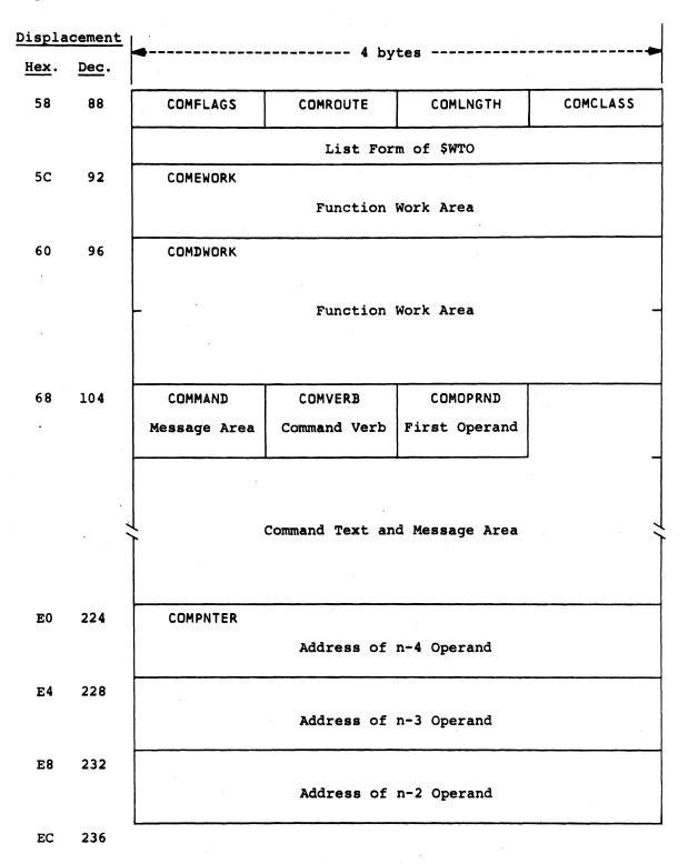
Figure 4.5.1 -- HASP COMMAND PCE WORK AREA FORMAT
