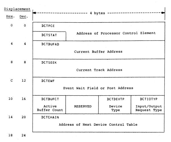
Figure 8.5.1 -- DIRECT-ACCESS DEVICE CONTROL TABLE FORMAT
