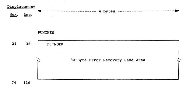
Figure 8.5.3 -- UNIT RECORD DEVICE CONTROL TABLE FORMAT (CONTINUED)
