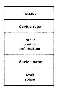
Figure 3.3.1 — The HASP Device Control Table (DCT)
