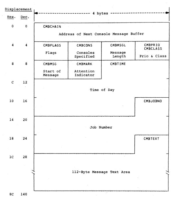
Figure 8.4.1 -- CONSOLE MESSAGE BUFFER FORMAT
